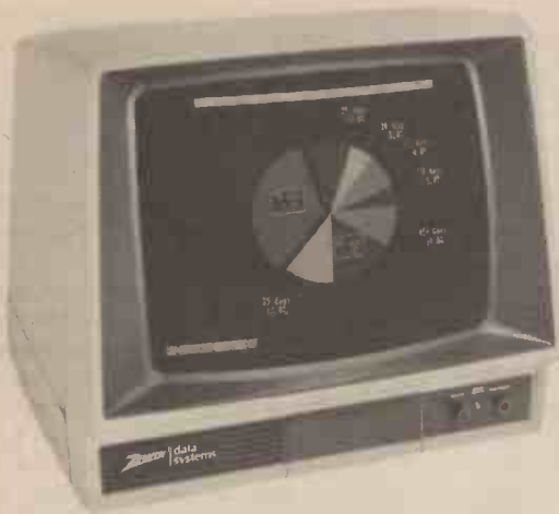
Model: Zenith ZVM 133 Screen: 13in. colour Input: RGB Resolution: not known Bandwidth: 20MHz Audio Output: no Price: £395 Notes: Tilt base available at £8, Commodore cable £6 Supplier: Zenith Data Systems Ltd., Bristol Road, Gloucester, GL2 6EE (0452 29451).
