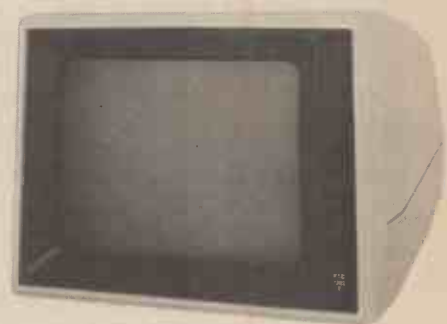
Model: Philips PTC1202 Screen: 12in. mono (green) Input: composite Resolution: not known Bandwidth: 22MHz Audio Output: no Price: £118 Notes: Also available, orange screen version at £99 Supplier: Swift Sasco Ltd., Box 2000, Crawley, Sussex (0293 28700).
