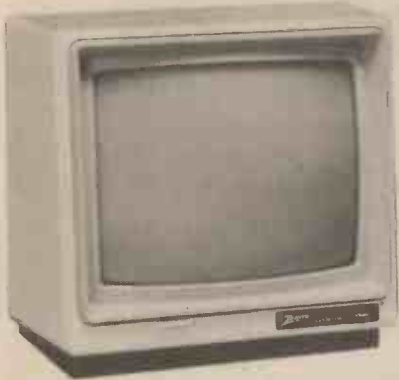
Model: Zenith ZVM-124 Screen: 12in. mono (amber) Input: TTL Resolution: not known Bandwidth: 22MHz Audio Output: no Price: £128 Notes: Tilt base available at £8, Commodore cable £6 Supplier: Zenith Data Systems Ltd., Bristol Road, Gloucester, GL2 6EE (0452 29451).
