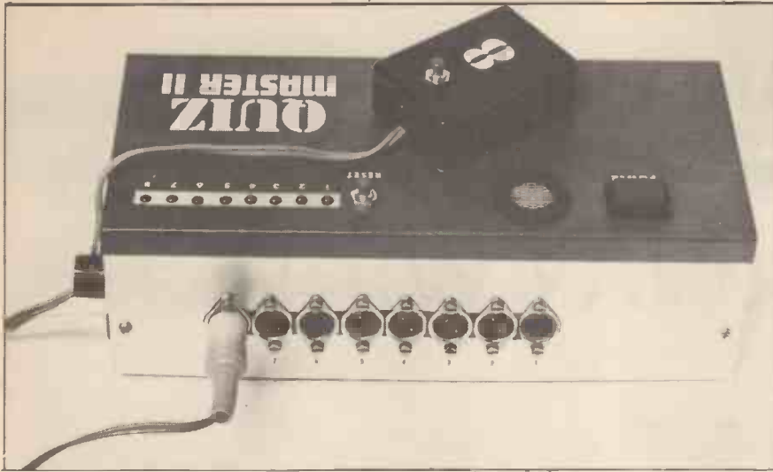
(Above). The rear view of the Quiz-Master II showing the DIN sockets with one response unit plugged in.
