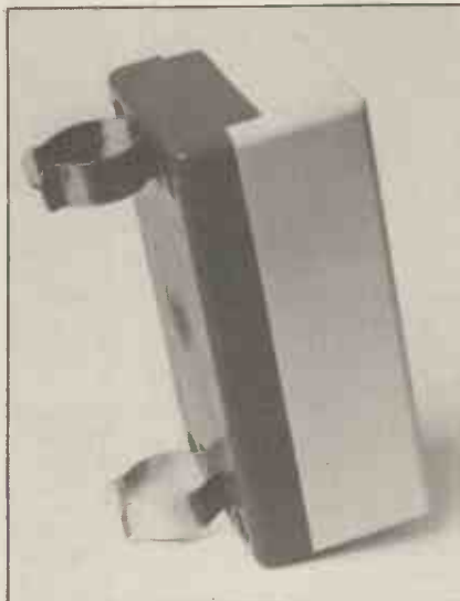
The prototype model showing how the spring clips protrude through two slots.
