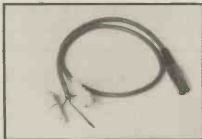
A "body" probe. The lint pads should be moistened with a saline solution.
