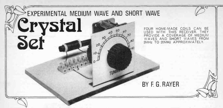
**T**HE POPULARITY of the crystal radio arises from its simplicity, and the fact that it needs no power supply. The circuit here allows for easy experiments with tuning, aerial and diode coupling, and frequency coverage. Wrong connections can cause no damage to any components.
