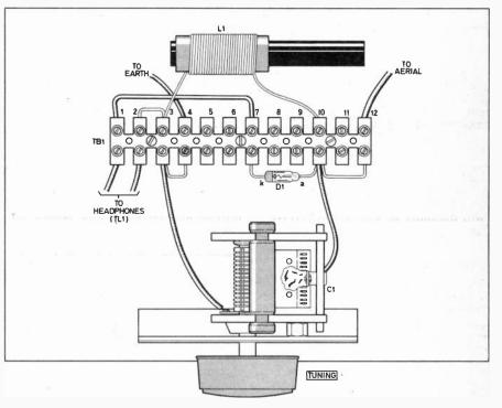
Fig. 2. Baseboard layout and interwiring for the crystal set.
