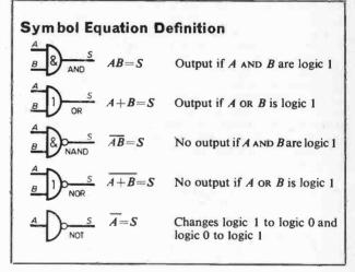
Fig. 7.3. The five basic logic gates and their definitions.
