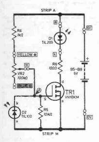
Fig. 2.16. Circuit for investigating the action of a light triggered switch.
