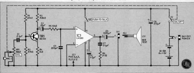
short periods of non-use with S1 left switched on. On the prototype S2 was a non-latching toggle switch mounted in the base of the box just in front of the handle so as to act like a trigger when in use.
