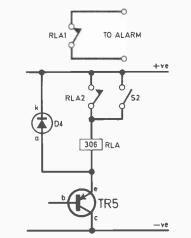
Fig. 6. The circuit can be modified to operate as a broken beam burglar alarm.
