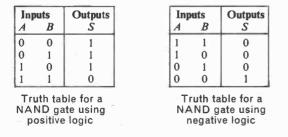
Once again it can be seen that the truth table for the NAND gate using negative logic is the same as the truth table for a NOR gate using positive logic.
