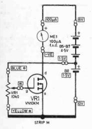
Fig. 2.10. Stage 2 of Experiment 2.2. Current flow through TRI for known VIN is being measured.
