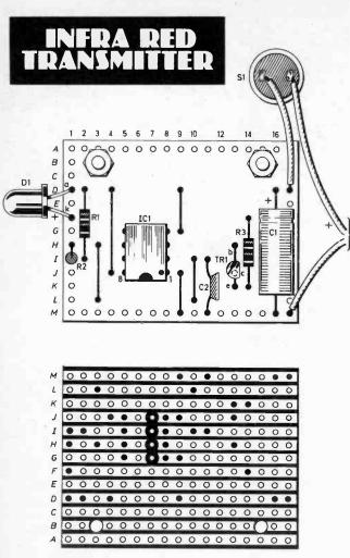
Fig. 3. Component layout and wiring details for the infra red transmitter.
