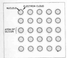
sides of the chip to a battery. The silicon is now a conductor. Substances such as silicon which can be conductors or non-conductors, depending on their temperature, are called semi-conductors.
