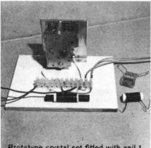
Prototype crystal set fitted with coil 1.
