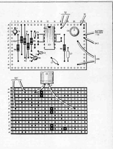
Fig. 3. Stripboard component layout showing trackbreaks on underside view. Note that C5 is mounted on underside of board.
