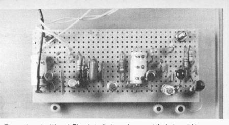
The receiver circuit board. The photo diode can be seen at the bottom right corner.
