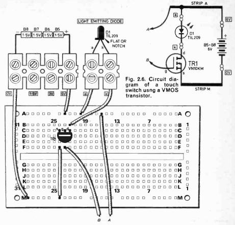
Fig. 2.7. The layout on the breadboard and interwiring for the circuit in Fig. 2.6.
