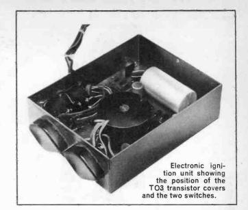
Also at this point any mounting holes for securing the unit to the car bodywork must be drilled ensuring that they will not be obscured by either the p.c.b. or the switches after the final assembly of the unit. The mounting holes for the switches and transistors TR1 and TR2 are shown in Fig. 7.
