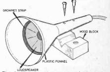
Fig. 2. Home-made version of the born speaker showing a suggested method of mounting.
