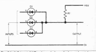
Fig. 7.6. A 3-input AND gate made from diodes and resistor.
