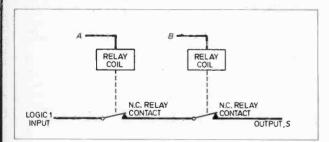
Fig. 7.1. A 2-input NOR gate realised using two normally closed relays connected in series.
