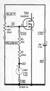
Fig. 2.8. Stage 1 of Experiment 2.2 to observe and measure the action of a MOSFET. Here we are calibrating V IN.
