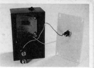
The transmitter with top panel removed. The "trigger" switch S1 is shown mounted on the top panel.
