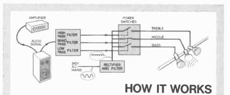
The audio signal is fed into the unit. It passes through an isolating transformer and is then split up into three frequency bands using simple RC filters.
