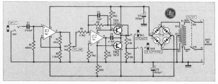
Fig. 1. Circuit diagram of the Guitar Practice Amplifier and its mains power supply.
