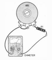
Fig. 4. Calibration circuit for VR1.
