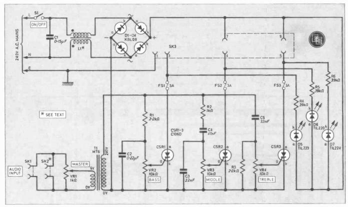
Fig. 1. (above) Full circuit diagram of the Three Channel Sound to Light.
