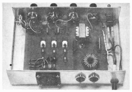
The front panel mounted components wiring is shown above and below the wiring to SK3 and other rear panel mounted components can be seen.
