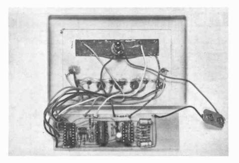
as far as possible avoid touching the pins when handling these devices. It is recommended that the interconnecting strip on the Soldercon pin be left intact until the i.c.s are mounted, and then snapped off.
