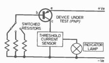
Fig. 2. Transistor tester with threshold current sensor.
