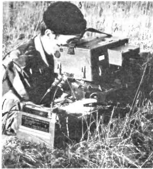
The Ferranti Laser Target Marker used by ground forces to designate targets to supporting, strike aircraft.
