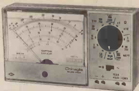
A modern example of a multimeter, having excellent ranges. One attraction is the use of a "mirror" scale.
