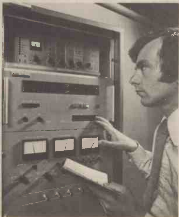
Modern radio communications exemplified by this Marconi drive unit and 1 kilowatt fast tuning transmitter.
