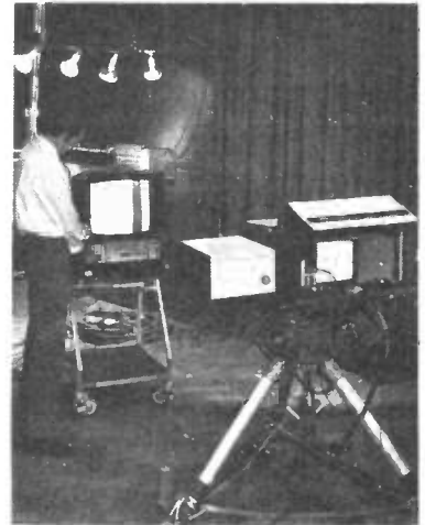
EMI colour TV camera and monitor as used in many TV studios.
