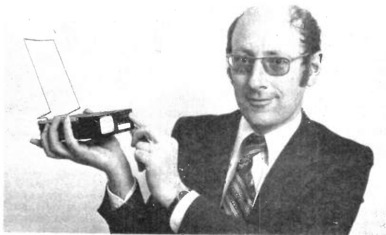
The set, with u.h.f. aerial raised, being operated by Clive Sinclair. A v.h.f. telescopic aerial is also fitted and provision has been made for connection to an external aerial.
