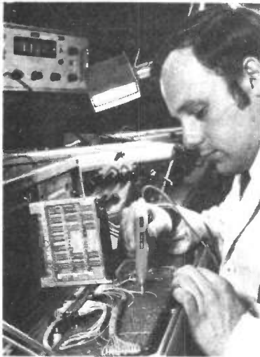
An EMI logic probe of the type supplied to the Royal Navy for checking out ship-borne data processing equipment.
