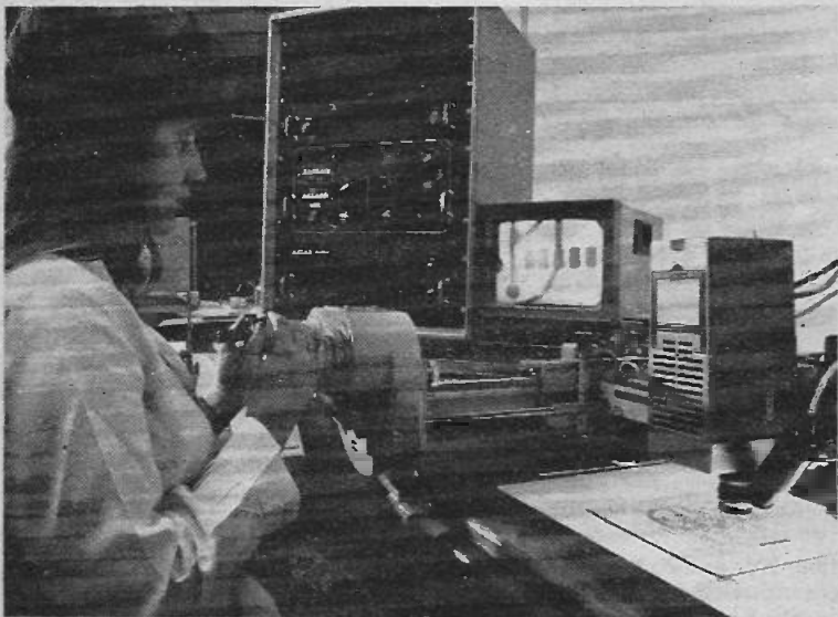
Training on an optical inspection machine. The operator is checking the positional accuracy of holes in printed circuit master artwork.
