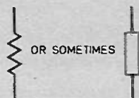
Fig. 1. 4a. Symbols used for representing a resistor in a circuit diagram.
