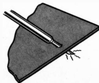
Fig. 1. Using a soldering iron to make small holes in plastic
