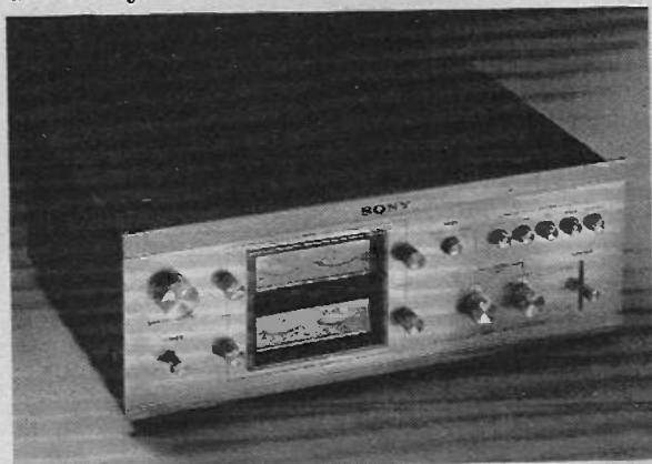
The Sony SQD2020 SQ matrix 4-channel decoder. Also handles CD4, regular matrix and stereo.
