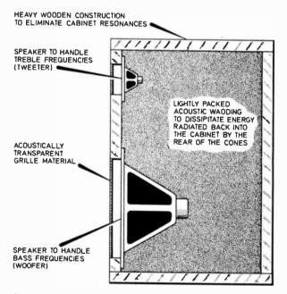
Cross sectional view of a basic speaker system employing two speaker "drive" units.
