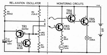
Fig. 2.2. The practical oscillator circuit. Transistors TR3, TR4 and TR5 do not affect the oscillator, they are used for monitoring purposes only.
