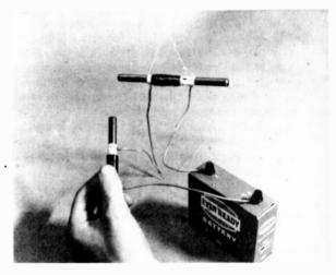
Fig. 3.4. Experiment for showing that like poles repel, unlike poles attract.
