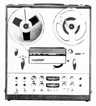
The Brenell Mk 6 stereo tape deck complete with pre-amplifiers but not power amplifiers or loud-speakers. This is a high quality hi fi tape unit.
