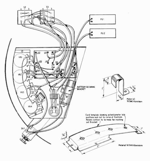
Fig. 20. The complete wiring details of the Beta "electronics". Screened cable *must* be used where indicated. The units are switched on by inserting the jack plug. Fig. 21. Details of the potentiometer fixing bracket and the battery securing bracket.
