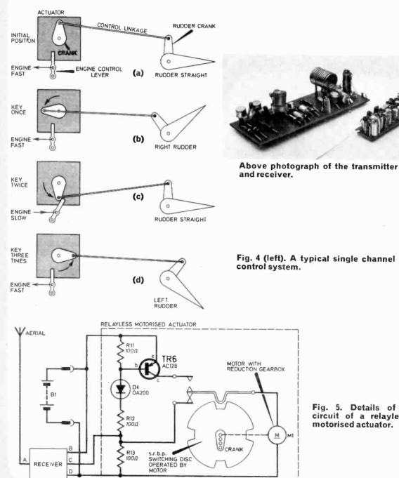
Fig. 5. Details of a circuit of a relayless motorised actuator.
