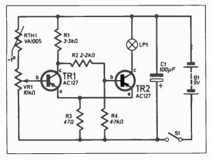
Fig. 1. Complete circuit diagram of the Ice Warning Device.
