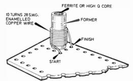
Fig. 3. Winding details for coil LI.
