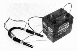
Fig. 3.2. Details of making the U-shaped electromagnet. A convenient supply is obtained by connecting two  $4\frac{1}{2}$  volt bell batteries in series.
