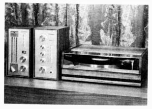
Individual hi fi units made by Goodmans. The units are a.m./f.m. tuner, amplifier and record deck.
