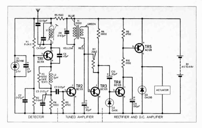
Fig. 1. The complete circuit diagram of the Radio Control Receiver.
