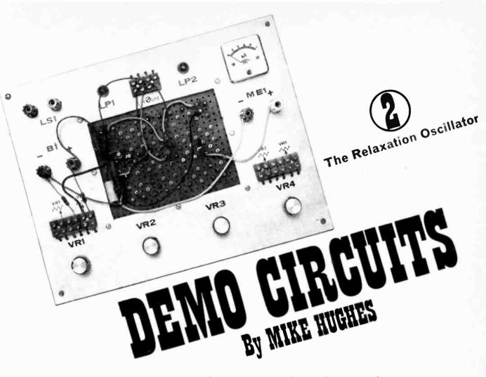
THIS month's circuit—shown in Fig. 2.1 belongs to a group called relaxation oscillators. The principle of operation is that C1 is allowed to charge up to a pre-determined value and then transistors TR1 and TR2 rapidly discharge the capacitor. The potential at point A thus rises from nearly zero to the pre-determined level following the characteristic capacitor charge curve and then reverts rapidly back towards zero.
