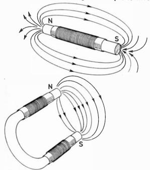
Fig. 3.6. Imaginary lines of force around (1) straight magnet (2) U-shaped magnet.
