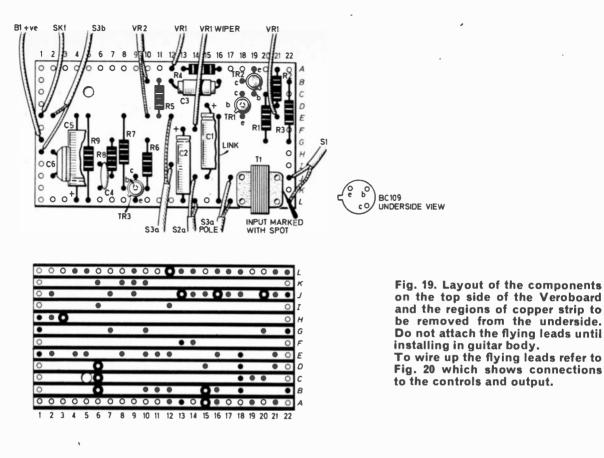
remaining cut-outs on the underside of the board as detailed in Fig. 19.
