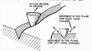
Fig. 1. Showing how a stereo signal is obtained from the record.
