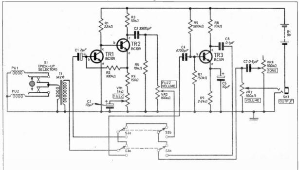
The two switches S2 and S3—both double-pole two-way types—are used for passing the resultant signal from the transformer through either fuzz or treble boost effects. For position of switches as shown, the signal passes straight to the output jack socket.
