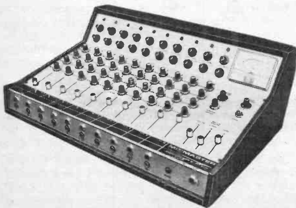
A ten-channel audio mixing unit with built-in "reverb". Each channel has its own tone controls and slider volume control. (above) The electronics within—its size and compactness is due to the use of semiconductors.
