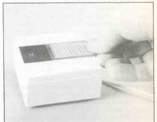
The correct wiping action to operate the lock.
