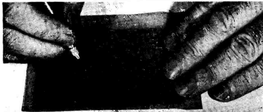
Fig. 7. Remove the unwanted film, leaving film over the areas where copper is to remain.
