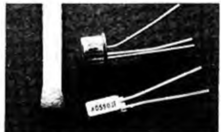
Tiny, what? The two versions of the AD590 packaging compared to a match head. Above is the H package (TO-52); below is the ceramic F package.
