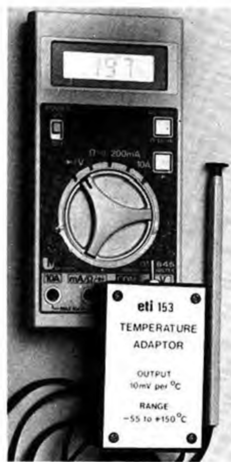
And it's 19.7^{\circ}\text{C} ! Our adaptor plugged into one of the lab multimeters
