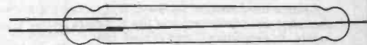
Fig. 5. This type of reed switch may be used for either change-over, or normally closed operation.
