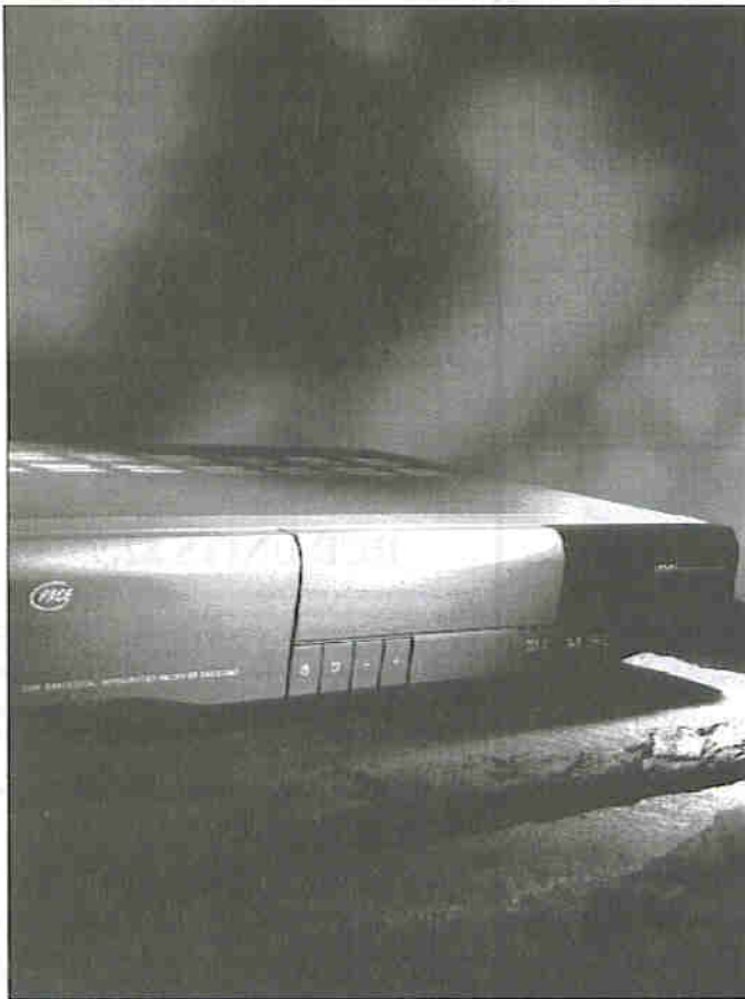
A digital integrated set top box carrying cable, satellite and terrestrial decoding: a serious piece of hardware
