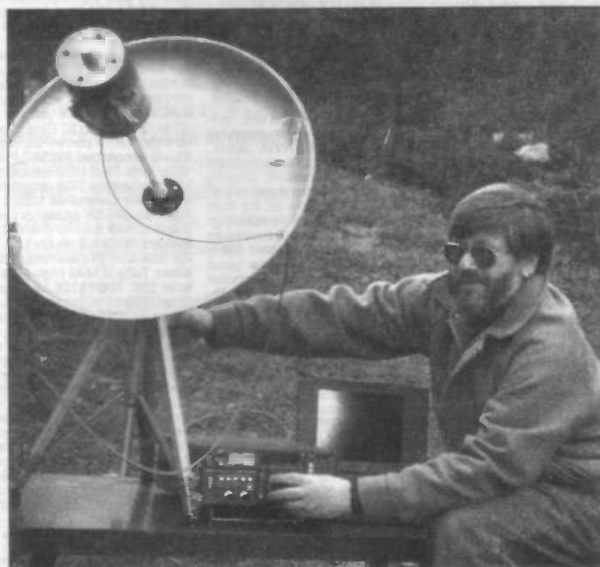
Dr. H. Paul Shuch attempts to measure sun noise with a portable radio telescope. This system serves as a test-bed for the hardware and software to be used for the Project Argus all-sky survey. The actual antennas used for SETI are much larger.
