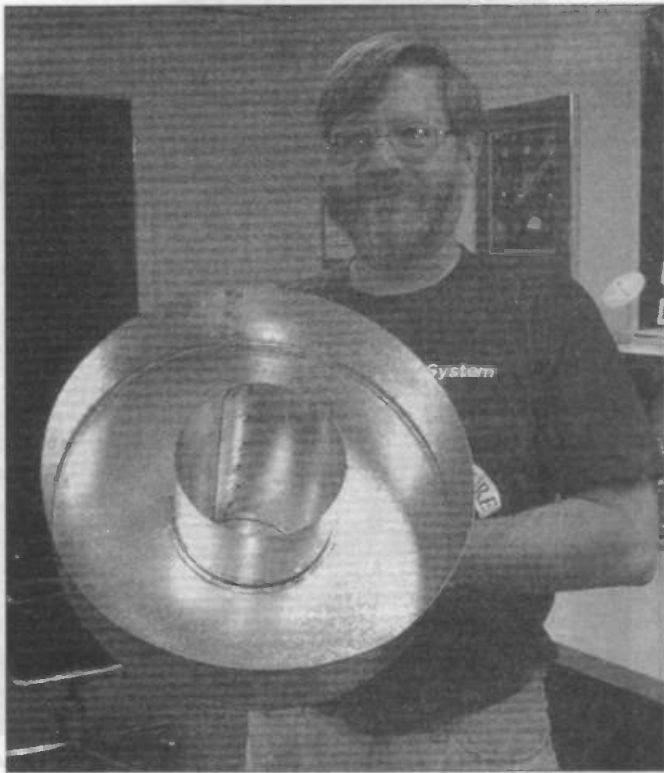
Improved SETI feedhorn incorporating a scalar choke ring. The position of the choke ring along the waveguide feedhorn can be varied to optimise performance for maximum gain, or minimum noise temperature, as the user requires. The feed can be readily optimised for dishes with a wide range of focal length to diameter (F/D) ratios.
