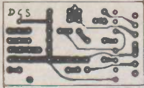
Field power supply foil pattern
