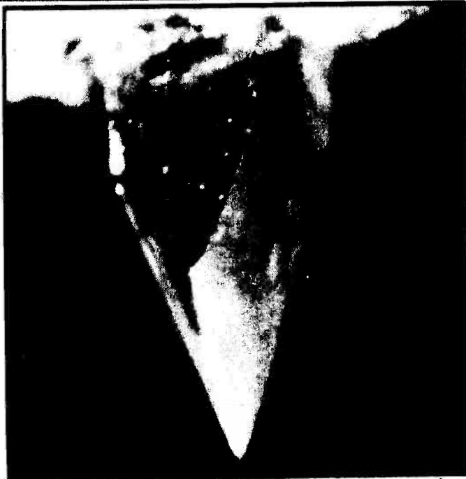
The point of the exercise? The van den Hul in close-up. The advantages of the shape are claimed to be decreased wear, due to increased contact radius, and improved groove following abilities.
