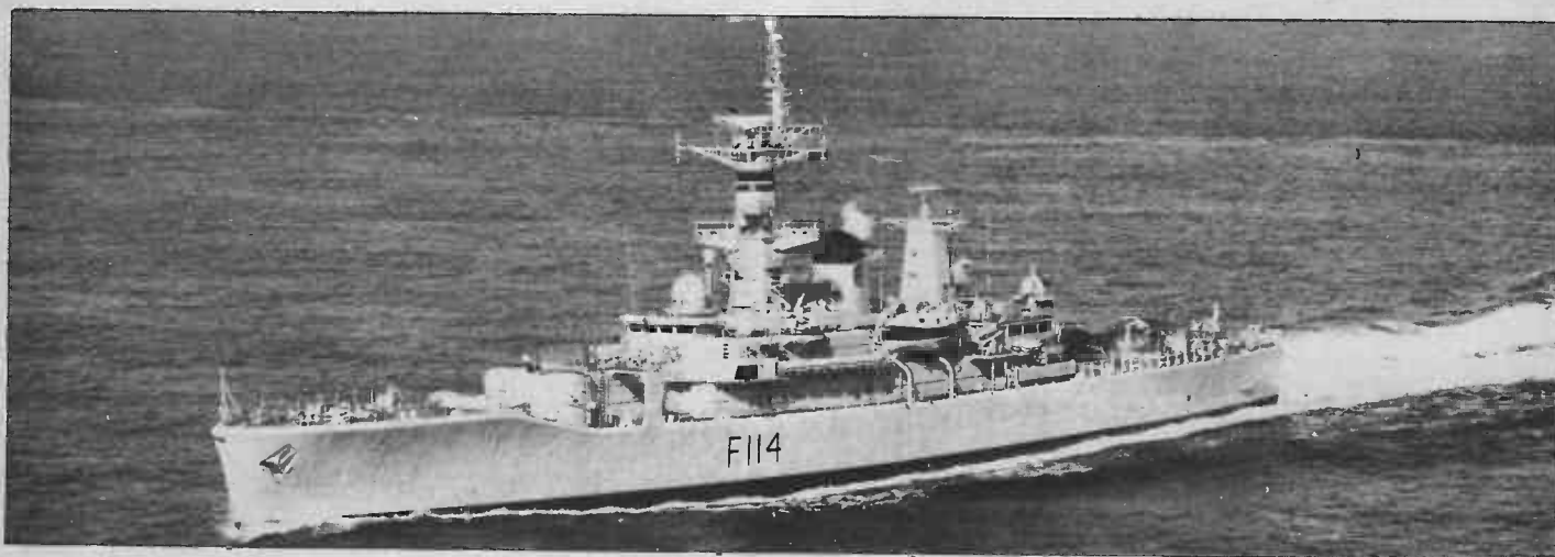
HMS Ajax is a Leander Class frigate with the Ikara ASW system and Seacat guided missiles.
