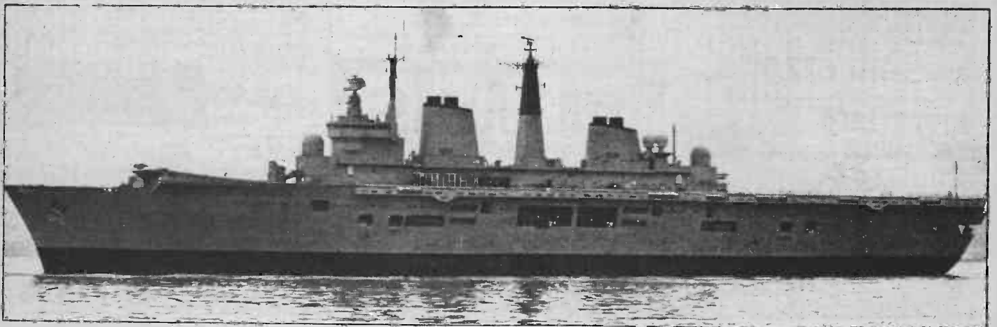
HMS Invincible, an ASW cruiser. The ramp near the bows is for launching Sea Harrier jump jets.
