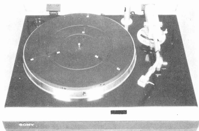
Sony PSX-75 bionic record deck. Note the pillar in the background and the prisms set into the turntable mat. These control record size indication.
