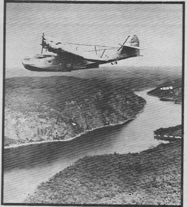
Photo 5. Catalina aircraft with em magnetometer system fitted.
