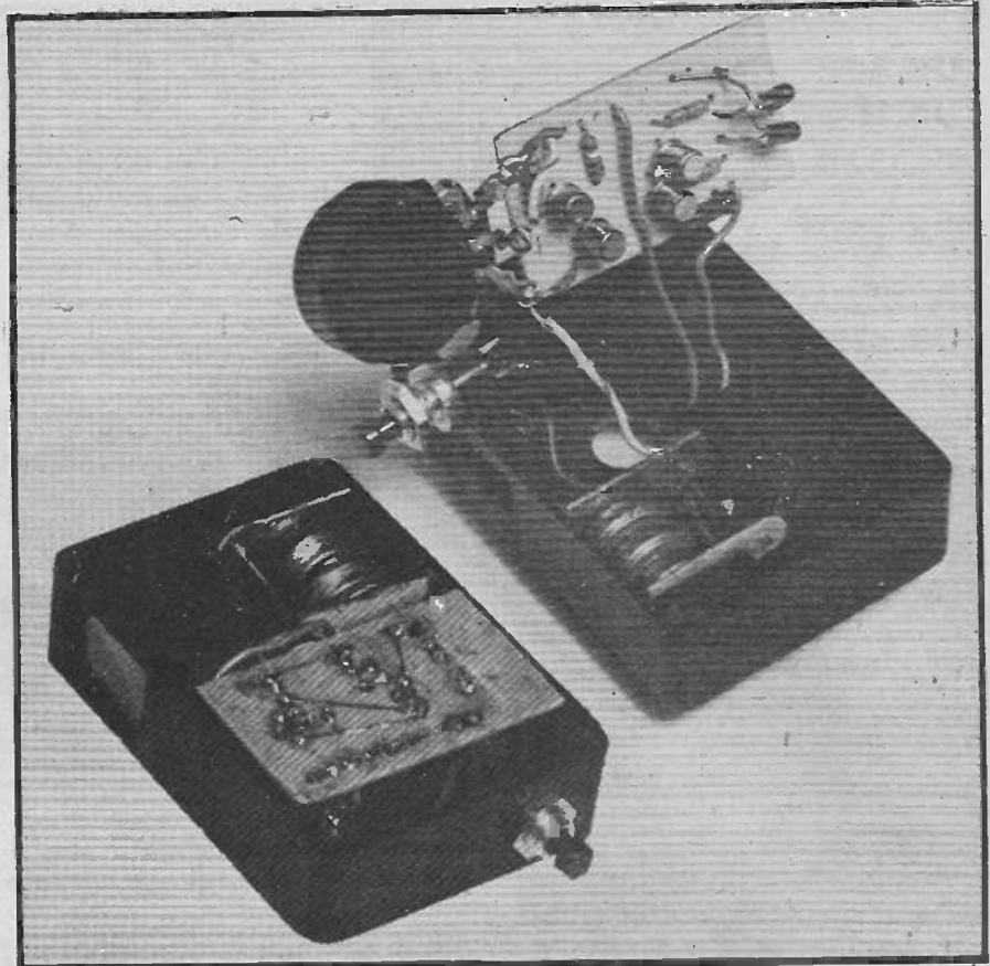
Inside the Mark II. The pcb is mounted on the back of the pot.
