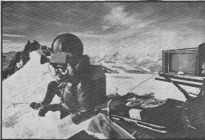
An Ampex BCC-2 portable colour camera was recently carried to the summit of the Dufourspitze, Switzerland's highest peak. The cameraman is also wearing the back-pack, through which this new hand-held camera generates full broadcast-quality pictures. Behind him is the dish of the temporary microwave link, and the Ampex VR-3000B portable videotape recorder is in the foreground with a monitor.
