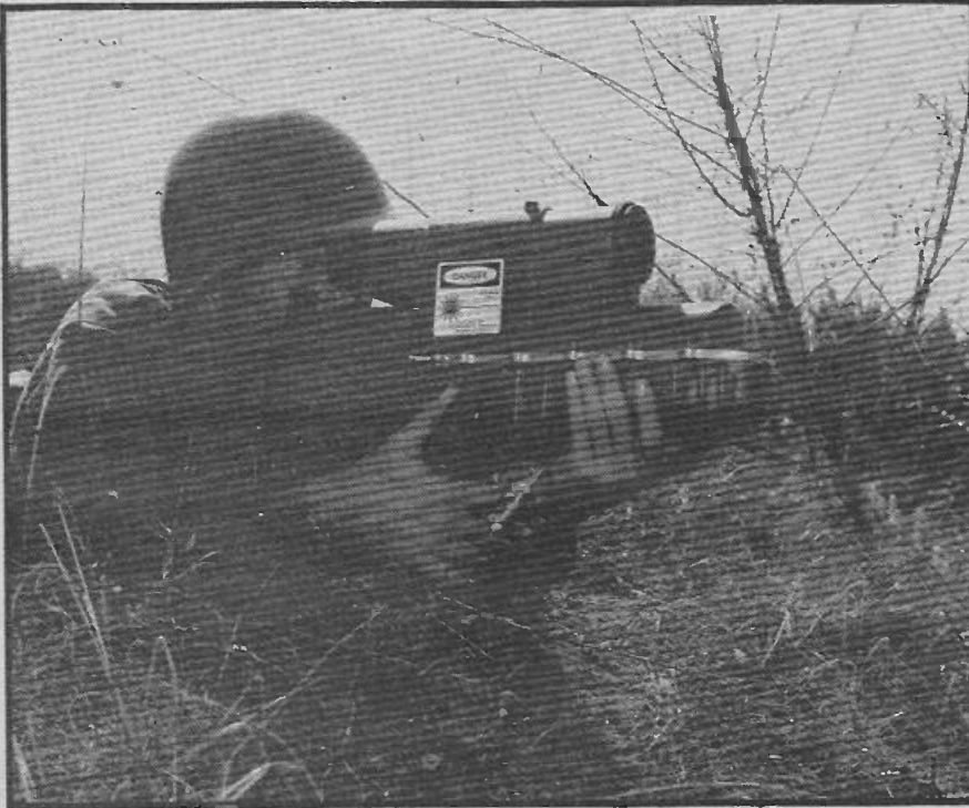
LASER GUN -- A lightweight laser gun, weighing only 13 pounds, can be aimed by infantrymen to pinpoint targets for laser-homing missiles and projectiles, or used to designate targets for airborne laser spot trackers. It is built by the Hughes Aircraft Company, which has delivered 12 development units to the US Army Electronics Command. Starting March 1, the US Army will begin a six-month programme to field test the equipment under actual operating conditions against a variety of laser seekers and laser spot trackers.
