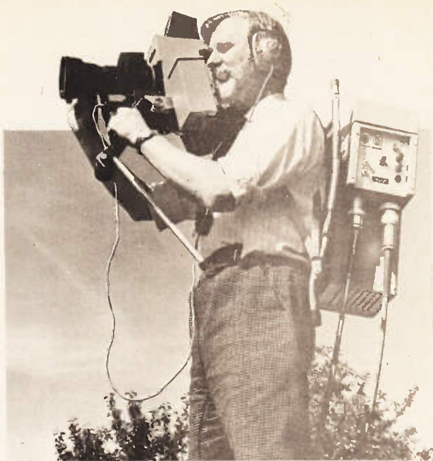
The portable version of the most advanced broadcast television camera, the Marconi Mark VIII. The camera is designed to produce high quality pictures which can be inter-cut with pictures from other studio cameras without degradation of picture quality. The Mark VIII Portable, which can be connected to a standard camera control unit, retains the features of automatic alignment and colour balance, particularly important for portable cameras which are subjected to very rugged treatment.
