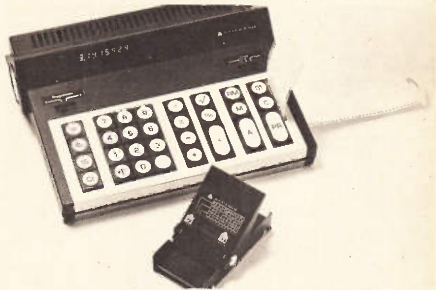
The new Advance programmable calculator showing the plastic strip programming device, together with the punch for writing programs.
