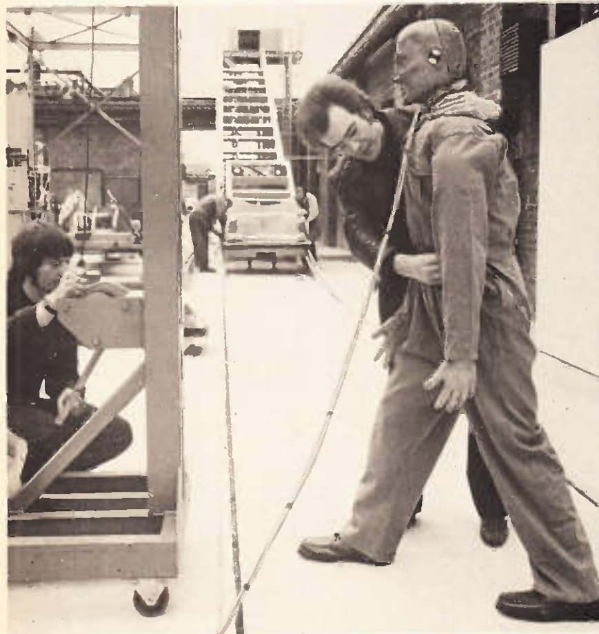
Fig. 14. Engineers set up a pedestrian dummy at the Rolls Royce test centre.
