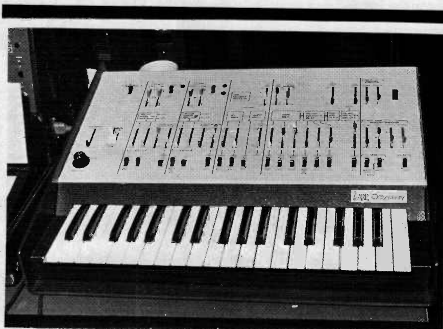
Fig. 12. ARP Odyssey synthesizer can route two keyboard voltages simultaneously to separate oscillators.
