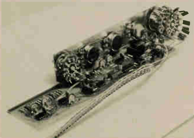
The voltage controlled oscillator, showing the assembly of board potentiometers and switches to the sub panel.
