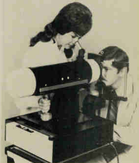
Fig. 4. Lining up the measuring system of the Ophthalmetron prior to carrying out a recording of the refractive error of the subject's right eye.
