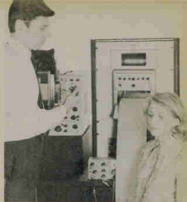
Fig. 9. Preparing to record an Electroretinogram; the subject wears a scleral contact lens containing one electrode, others being placed on forehead and ear. To the left of the picture an oscilloscope with a Polaroid camera attached provides a more detailed analysis of the ERG. The small unit in the centre is a high gain differential amplifier.
