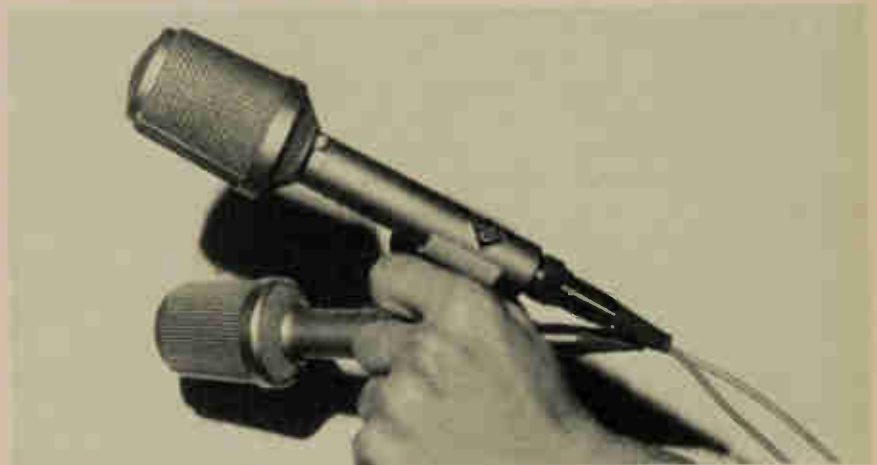
Crossed pair of Neumann KM 76 capacitor microphones — variable patterns set to cardioid — for location stereo recording.
