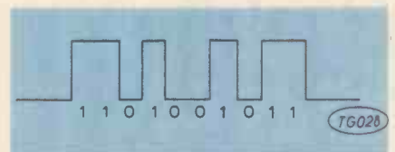
Fig. 2. The number 843 can be represented in a binary code by the train of pulses shown here.
