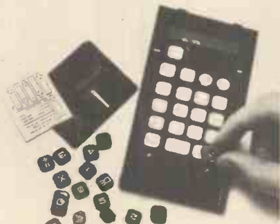
There's simple key loading and battery hatch assembly.
