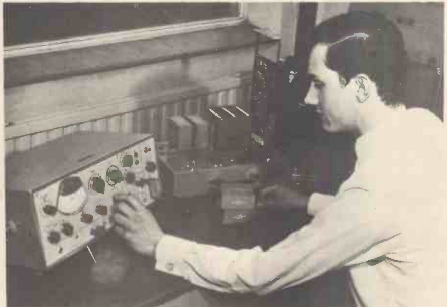
A Post Office regenerator type 2A undergoing a pre-installation check with a Marconi TF2342 regenerator tester.
