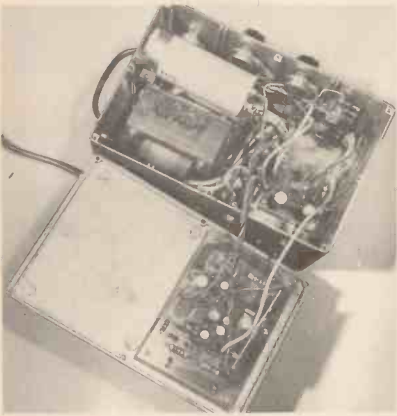
The preamplifier is mounted in the bottom of the existing power amplifier and the controls and input sockets on the right-hand side.
