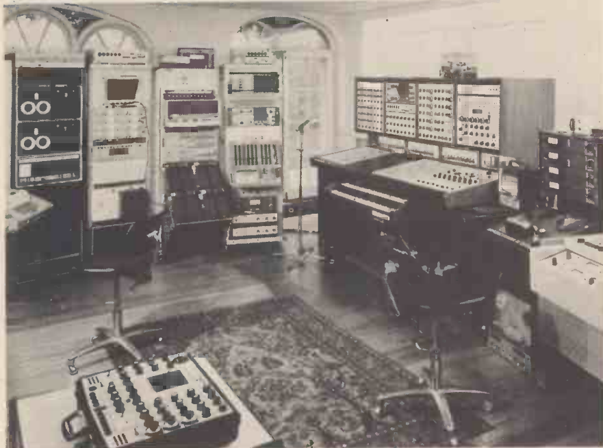
The Ultimate in Creative Capability? — the computerised Electronic Music Studio belonging to Peter Zinovieff (a director of E.M.S. (London) Ltd.) Note the recorders on the right of the picture — a 4-track Ampex, a stereo Revox (beneath the Ampex) and a stereo Philips Console Machine. In the background is a PDP8 computer which can interface directly with the music synthesiser to its right.
