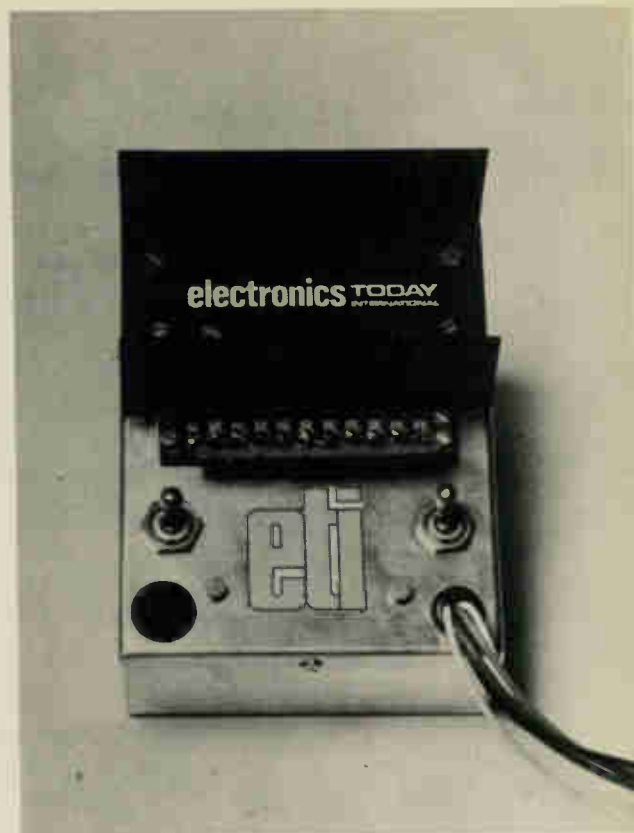
The completed unit. The heatsink should be sprayed matt-black.
