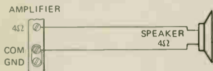
FIG. 1—SINGLE PA SPEAKER is connected like this. Just match the two impedances.
