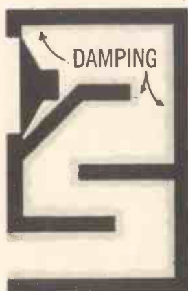
This sketch shows the original labyrinth designed by Olney in 1936. It was produced commercially by Stromberg Carlson for some years. The labyrinth behind the speaker damped its resonance and the auxiliary port near the bottom of the unit augmented its bass output.
