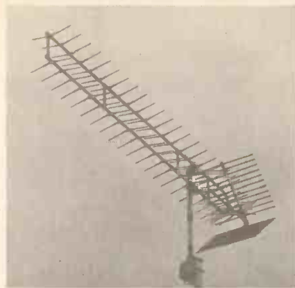
A number of companies specialise in high gain aerials; the one shown here is the Zodiac 30 from R. Smith Aerials of Luton. On Group A this gives more than 20dB gain.
