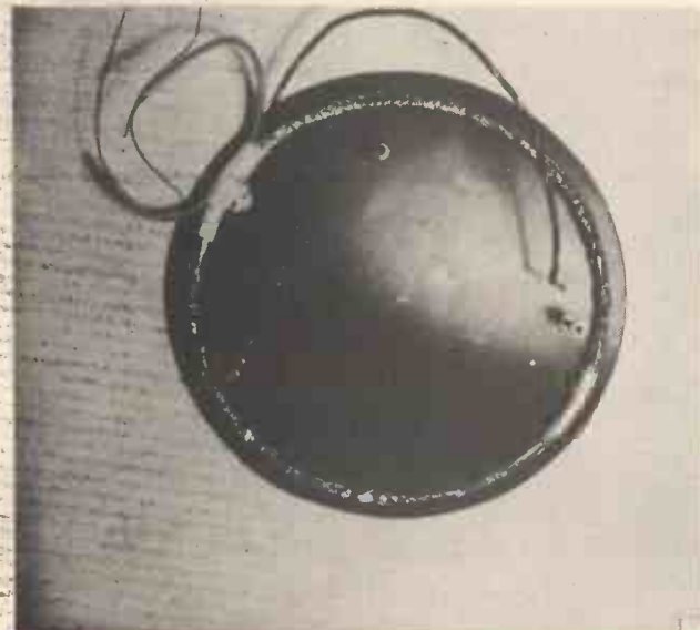
When screened the coil should be glued to the paxolin disc.
