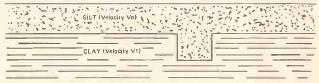
Fig. 3. Experimental refraction plot over a trench filled with silt.
