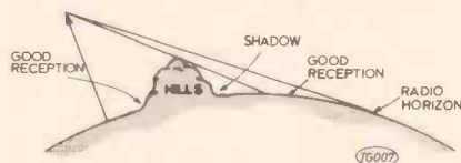
Fig. 2 The effect of hills on transmitter coverage.
