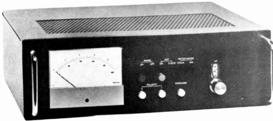
Miles Hivolt's TH25/25 can be switched on/off locally or remotely, and the voltage controlled manually or, by a low-voltage input, remotely. DVM readout of voltage and current provides remote monitoring.
