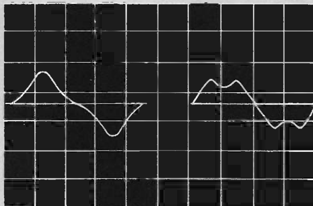
Fig. 16. These two distortion waveforms are alike except for relative phase relations.
