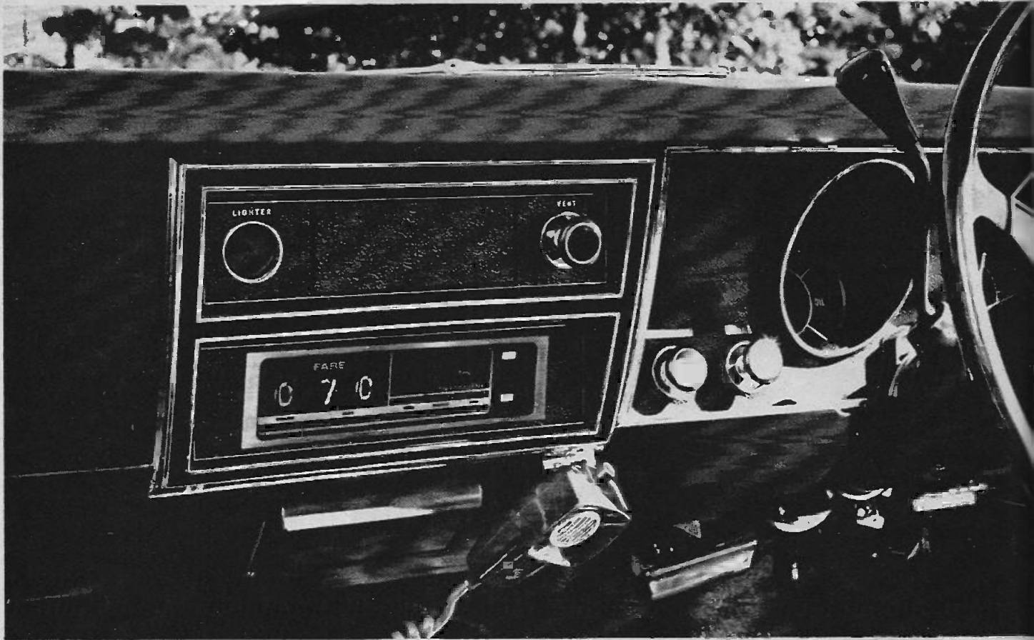
Electronic taximeter is located in car radio aperture.
