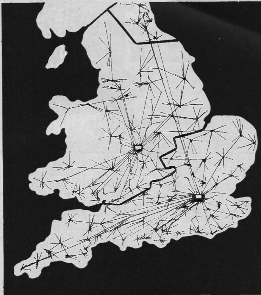
Fig. 3 Information is transmitted between branch offices and the London or Birmingham Computer Centres. This schematic map shows how branch terminals and centres are linked by telephone line.
