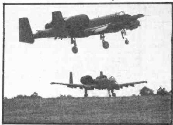
Below: Probably the ugliest aircraft flying. The A10 anti-tank craft. Note that because the engines are where they are from the ground they are hidden from next seeking missiles.
