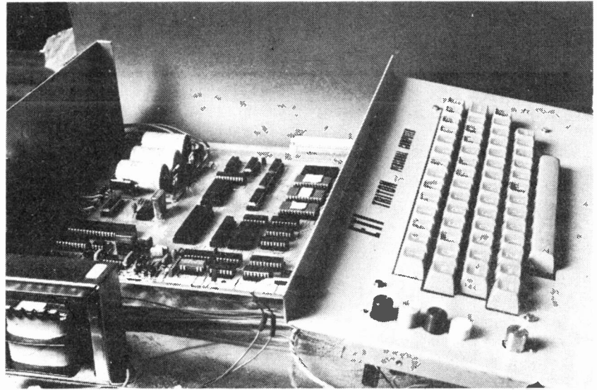
The Triton's board mounted in its case. Note that the extender socket is available on the right hand side of the case and that the output of the modulator is brought out to a UHF socket on the back panel. The back panel also carries the DIN sockets and the mains fuse.
