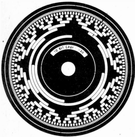
Fig. 4. A 10 bit optical Gray code disc. The value read from this gives the angular displacement.
