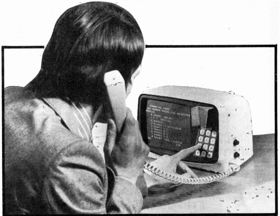
How a Viewdata receiver might be used. In the current experiment 200 pages are available. This prototype design — one of many — incorporates the 'phone with the receiver probably useful in commerce. Domestic installations are unlikely to incorporate the two as only a simple wire need be run from the phone's junction box to the TV.
