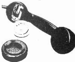
This telephone insert looks pretty standard. In fact it contains an FM radio transmitter with a range of several hundred metres
