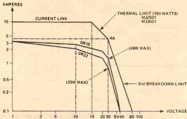
Fig. 6 Safe operating area curve for MJ2501/3001 and output current/voltage limits for PSU.
