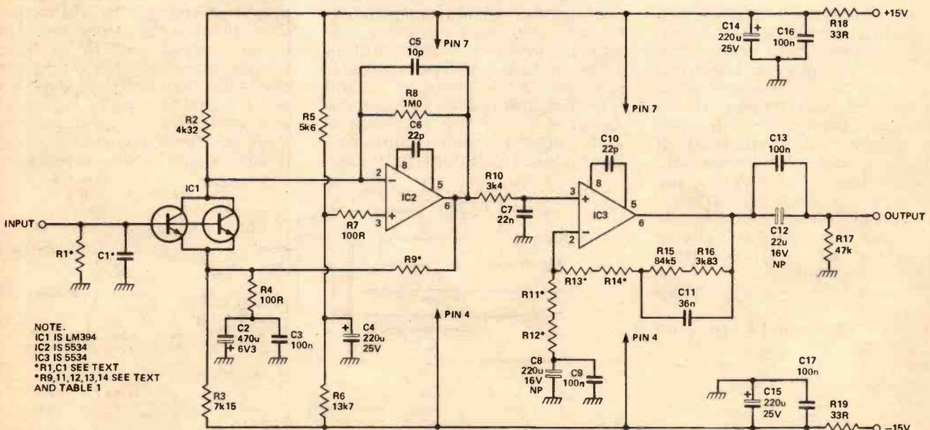
Fig. 2 Circuit diagram of the disc preamplifier stage.
