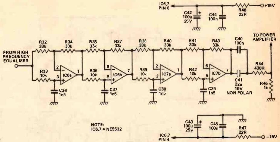
Fig. 11 Delay circuit.
