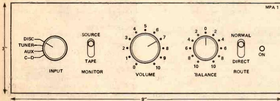
Fig. 5 A suggested front-panel layout for the small preamplifier.
