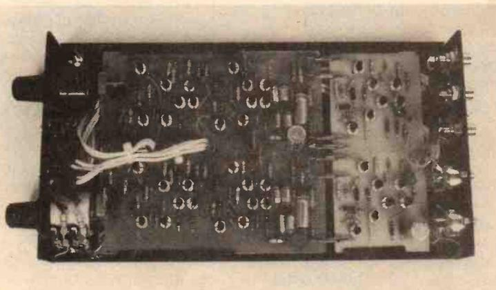
Inside the prototype preamplifier. Construction is on two boards, the main preamp module A-PR and the smaller input module. The latter is connected to the main board and the phono input by gold-plated connectors. This enables different input modules to be easily
