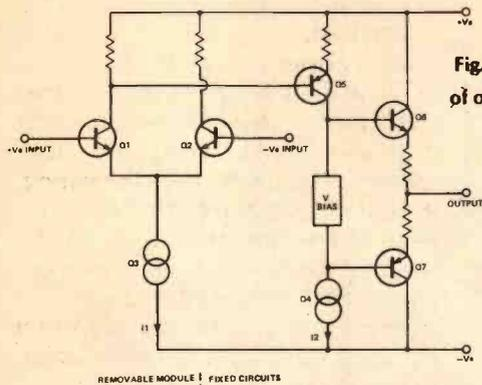
Fig. 1 Simplified diagram of one gain stage.
