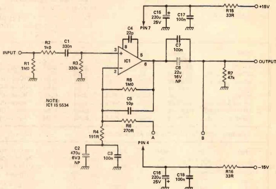
Fig. 4 Circuit diagram of the unbalanced output stage.
