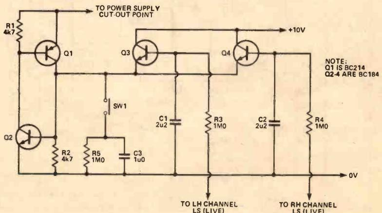
Fig. 3 Amplifier output DC detection and trip circuit.
