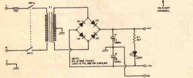
Fig. 4 Circuit diagram of the A-PSU preamplifier power supply.
