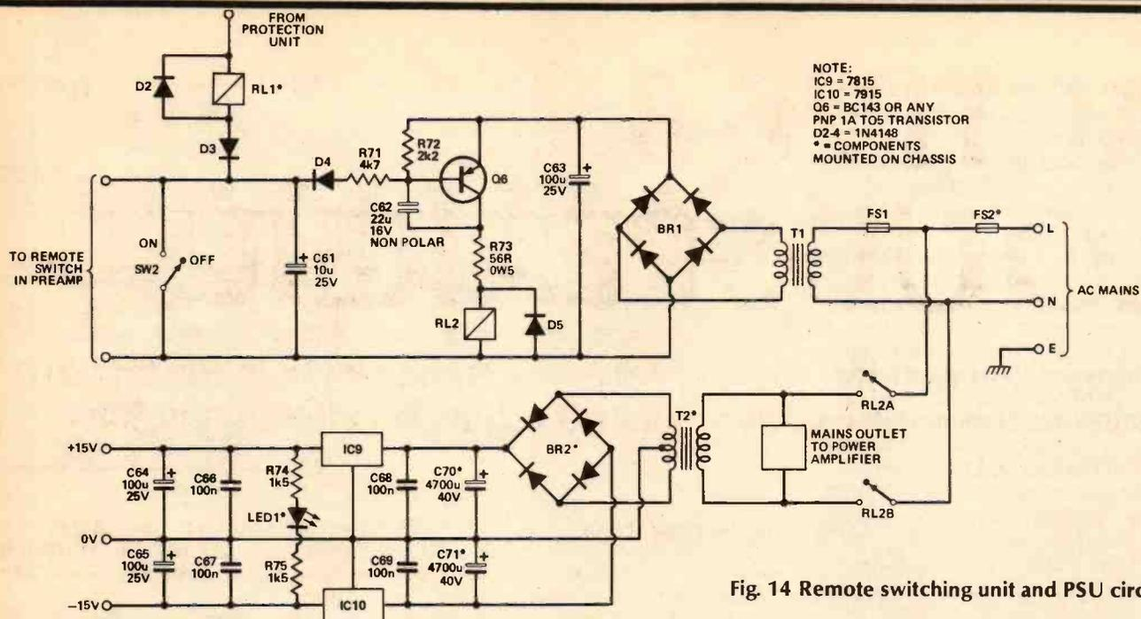
Fig. 14 Remote switching unit and PSU circuitry.
