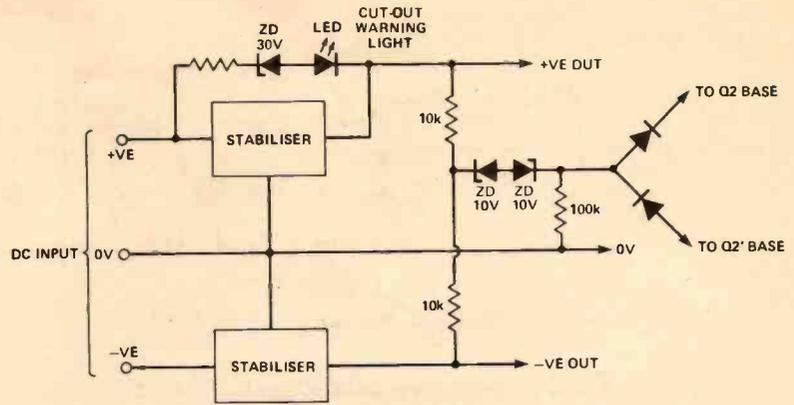
Fig. 4 Method of making both power supplies cut out simultaneously.
