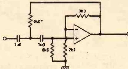
Fig. 4 Circuit for a second-order filter.
