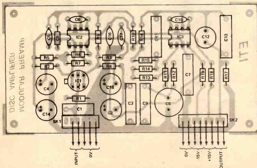
Fig 3 Component overlay of the disc amplifier PCB.
