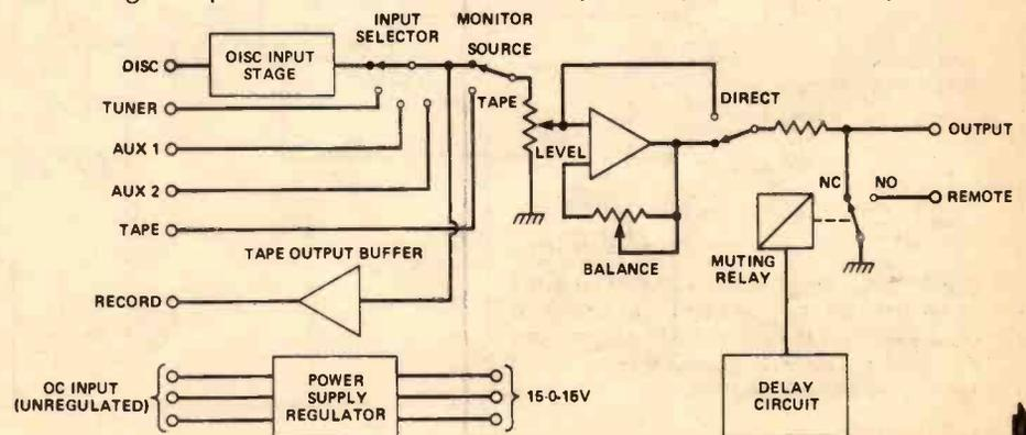
Fig. 1 Block diagram of the basic preamplifier.
