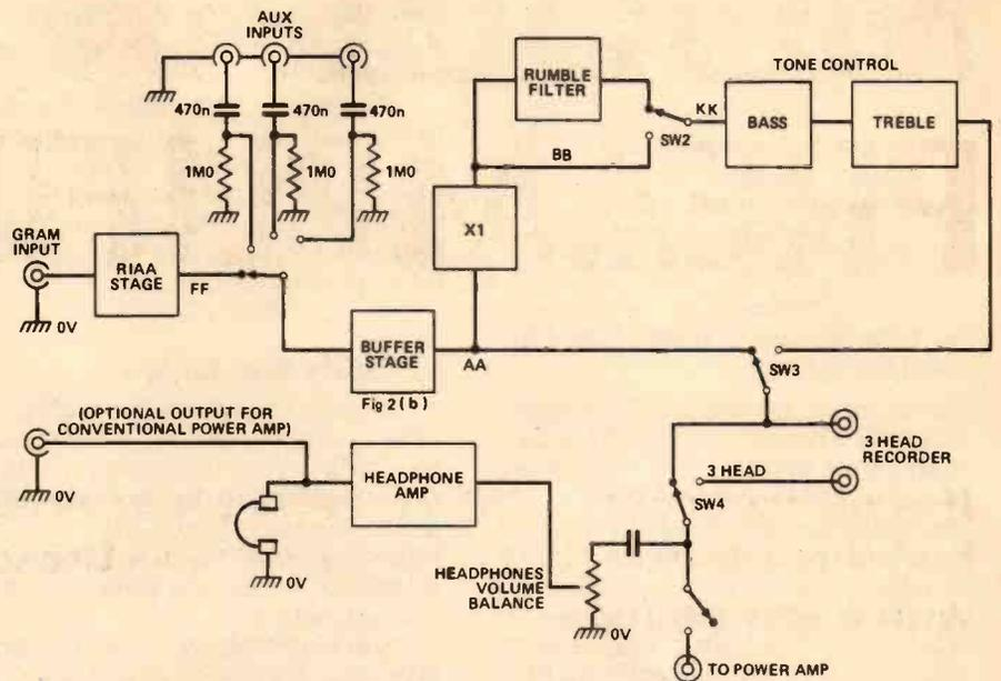
3 Alternative lay-out of preamp using discrete component buffer stage.
