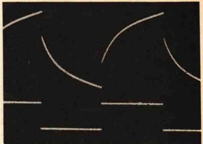
Response of the series feedback equalisation stage to a square wave input signal.
