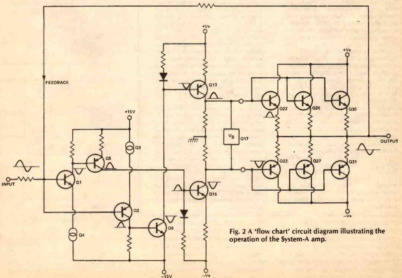
Fig. 2 A 'flow chart' circuit diagram illustrating the operation of the System-A amp.
