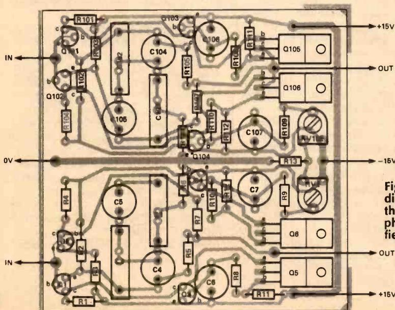
Fig. 11 Overlay diagram for the headphone amplifier.
