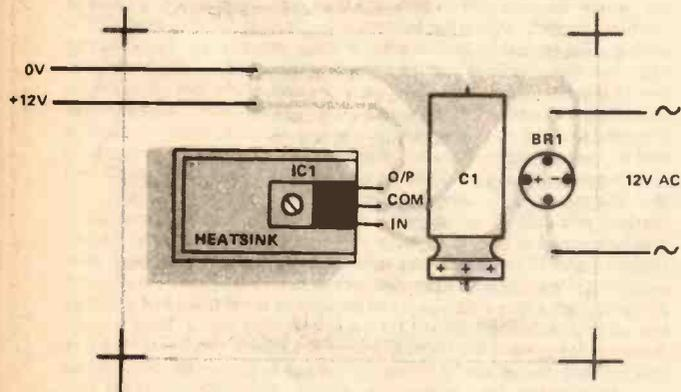
Fig.8 (above) Component overlay of the PSU.
