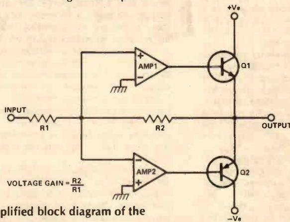
Fig. 1 Simplified block diagram of the power amp.
