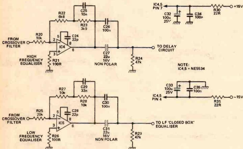
Fig. 9 Equaliser section circuitry.
