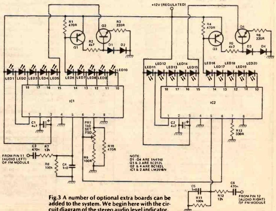
Fig.3 A number of optional extra boards can be added to the system. We begin here with the circuit diagram of the stereo audio level indicator.
