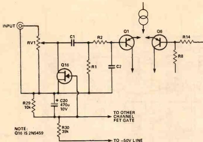
Fig. 11 FET input clamp circuit.
