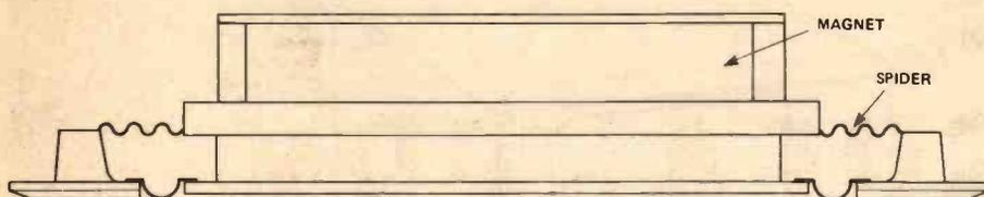
Fig. 1 Vertical cross-section through the Musician drive unit.
