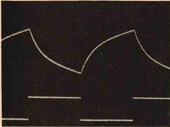
The response of the same stage when wired for shunt feedback.
