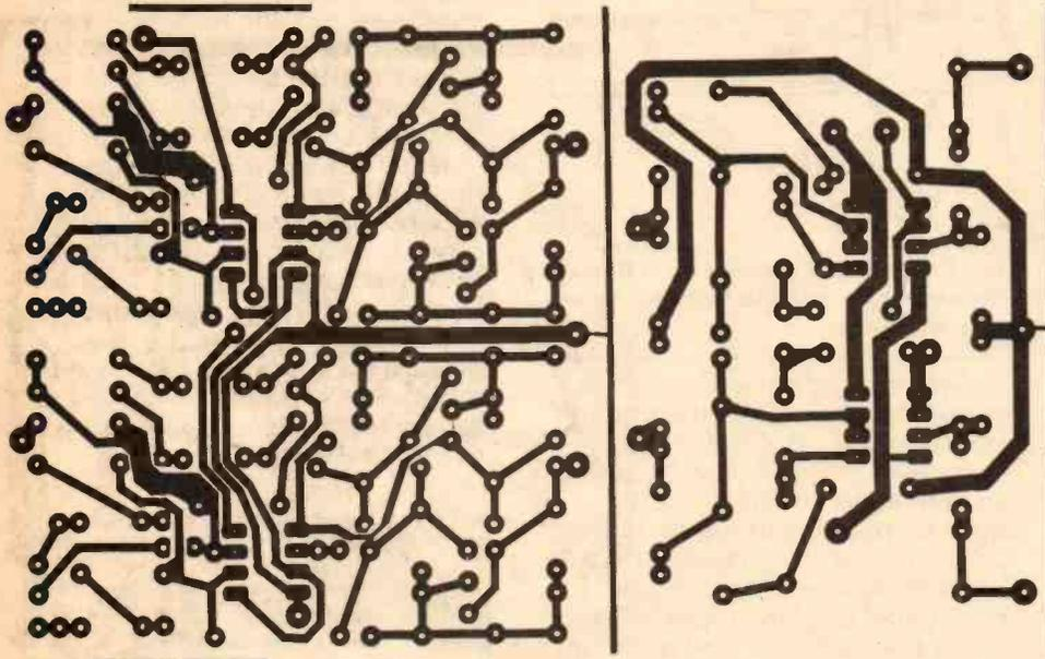
All the boards on these two pages are for the John Linsley Hood Audio Design Amplifier; all the corrections noted in the PCB overlay captions have been made on these boards.
