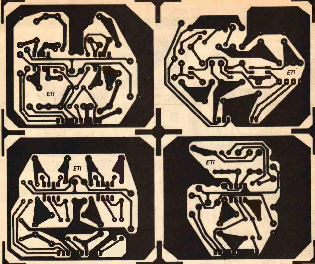
Above: the four plug-in modules for the Active 8 loudspeaker.
