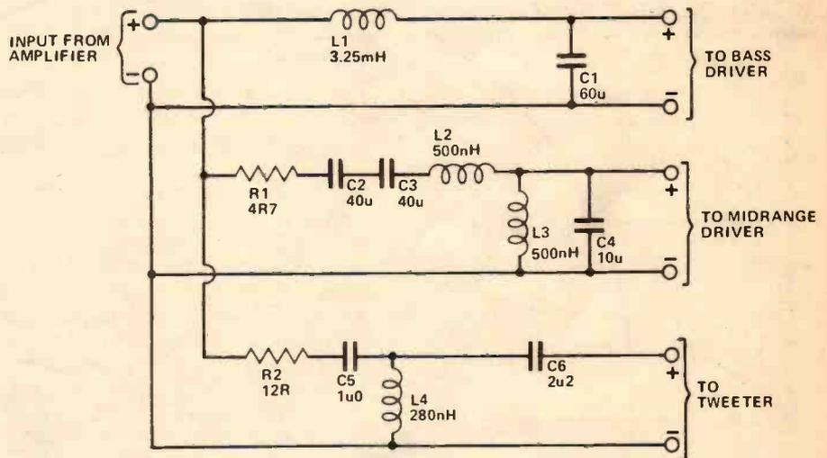
Fig. 6 Circuit diagram of the crossover.
