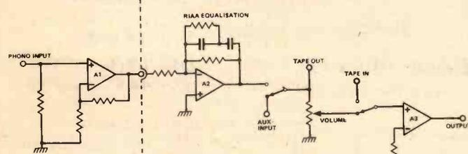
Fig. 2 Preamp block diagram. The 'op-amps' A1-3 are, in fact, built using discrete components.
