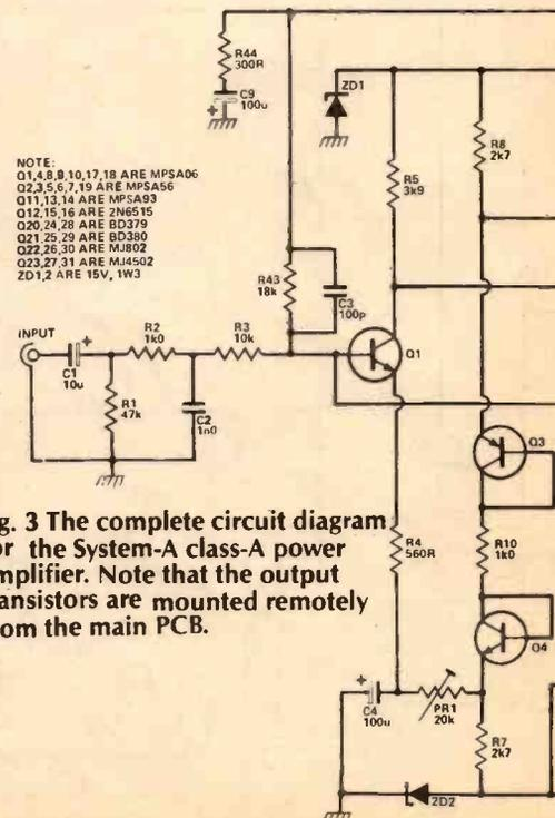
Fig. 3 The complete circuit diagram for the System-A class-A power amplifier. Note that the output transistors are mounted remotely from the main PCB.
