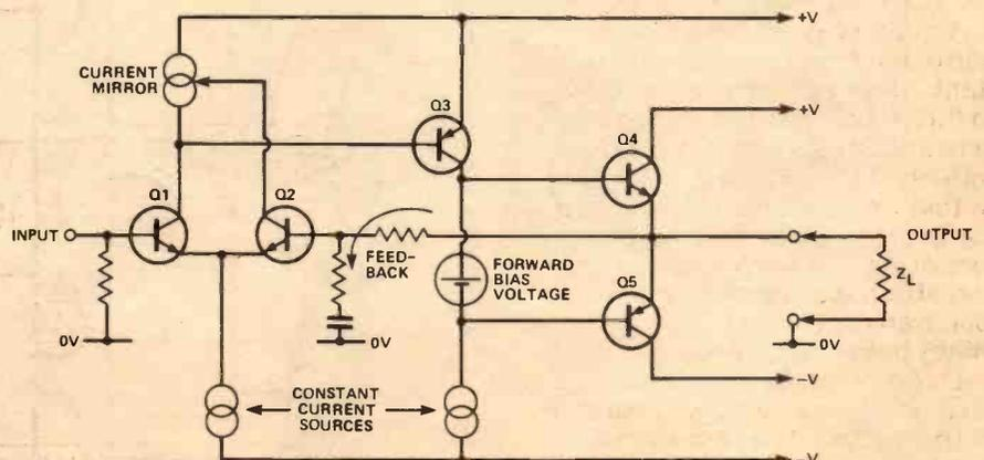
Fig. 1 Simplified structure of audio amp circuit.
