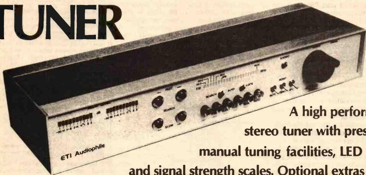
A high performance stereo tuner with preset and manual tuning facilities, LED tuning and signal strength scales. Optional extras are an automatic search-and-lock tuning facility and a stereo LED audio level indicator. Design by Ray Marston. Development by Steve Ramsahadeo.
