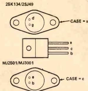
Fig. 1 The pin-outs of some of the off-board transistors.
