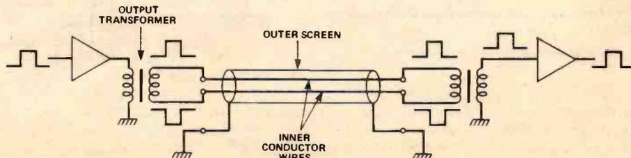
Fig. 4 The basic principle of balanced line operator.
