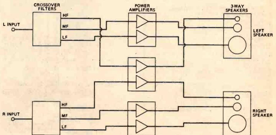
Fig. 3 Suggested set-up for a tri-amped system.
