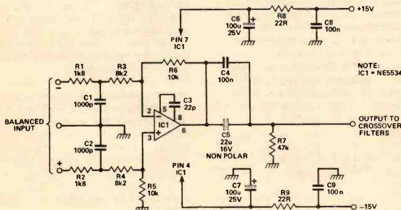
Fig. 3 Circuit diagram of the balanced input buffer.
