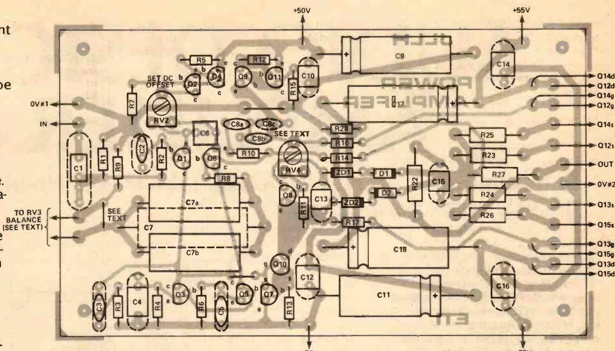
Fig. 7 The recommended PCB layout. Please note that the 'c' and 'e' labels on Q9 are reversed. The underlying PCB pattern is missing the link between the cathode of 2D1 and R16, RV4 wiper etc. This has been corrected on the foil pattern reproduced elsewhere in this issue, and on the board supplied by our PCB Service.
