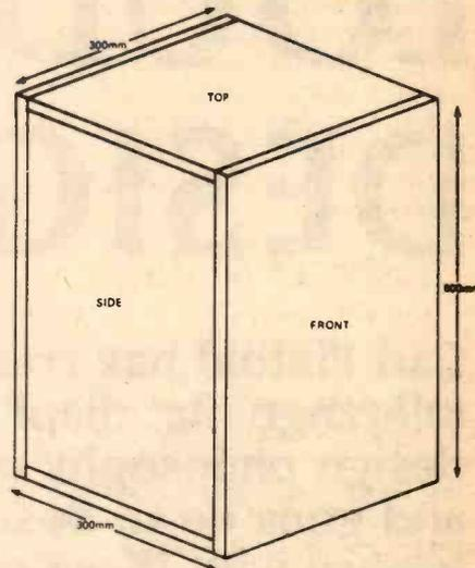
Fig. 10 This is how the panels fit together — if you did your sawing right!
