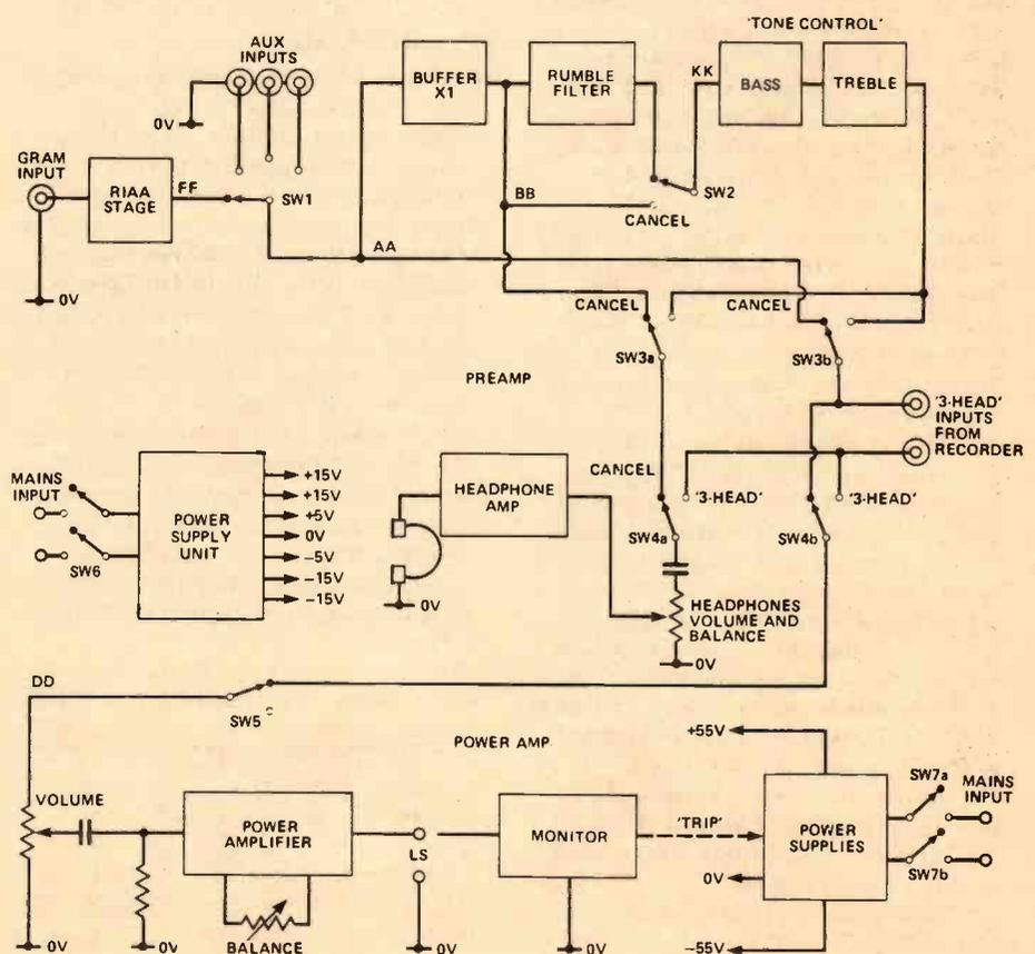
Fig. 1 Layout of the pre-/power amp system.
