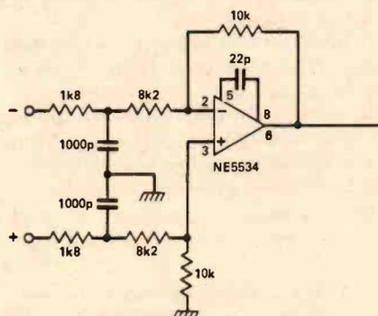
Fig. 7 A possible balanced input arrangement.
