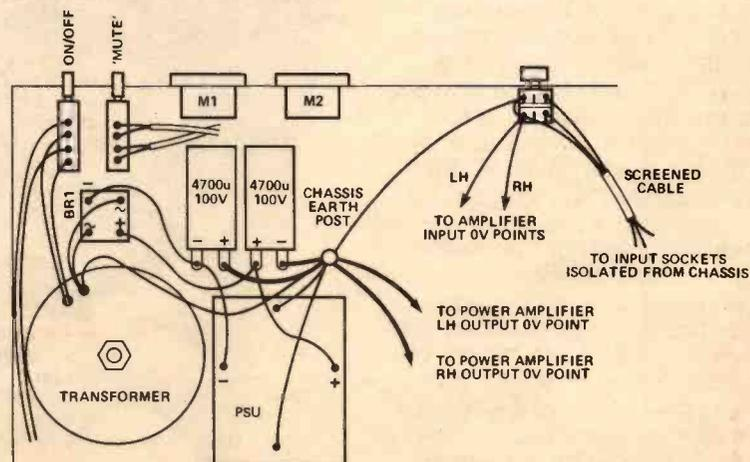
Fig. 8 Suggested lay-out of earth (0V) wiring for power amplifier and power supplies.
