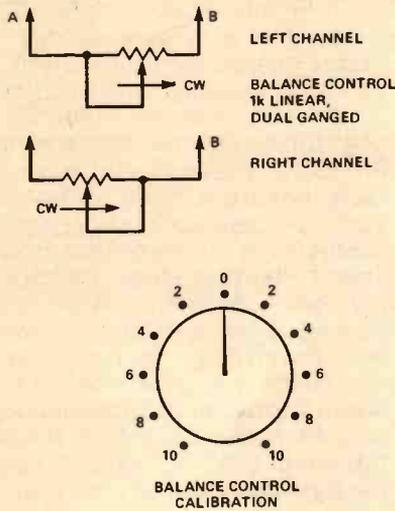
Fig. 6 Balance control connections and calibration.
