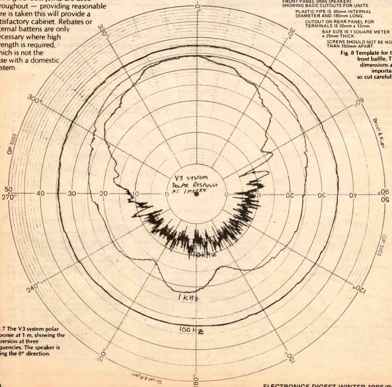
Fig. 7 The V3 system polar response at 1 m, showing the dispersion at three frequencies. The speaker is facing the 0° direction.
