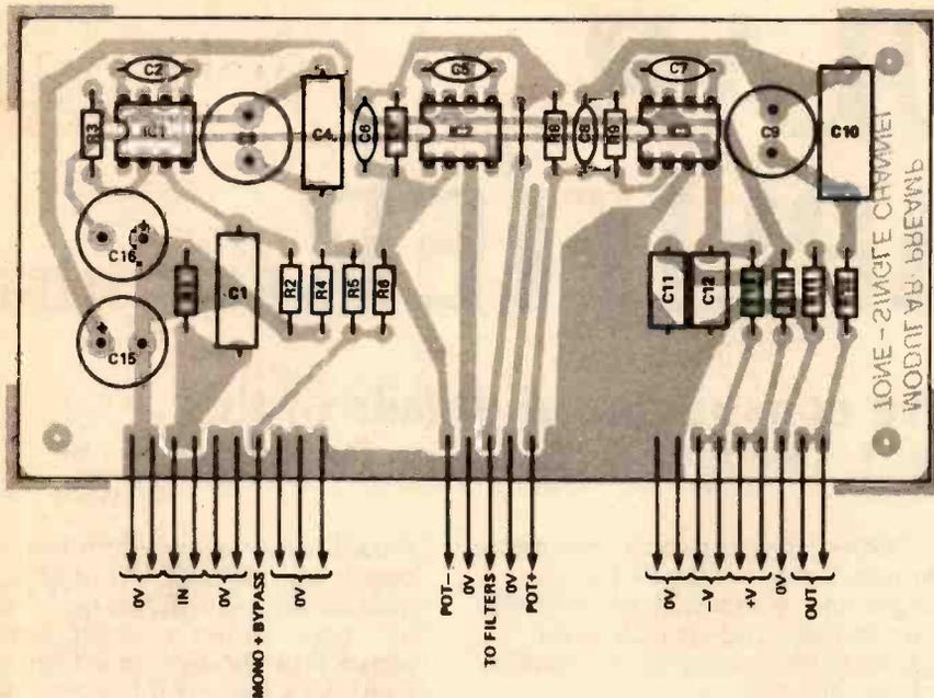
Fig. 1 PCB overlays for the tone control: the main board above is for a single channel, so two of these are required, whilst the filter board (below) is a stereo board, so only one of these is required. Note carefully which parts you need two of for stereo.
