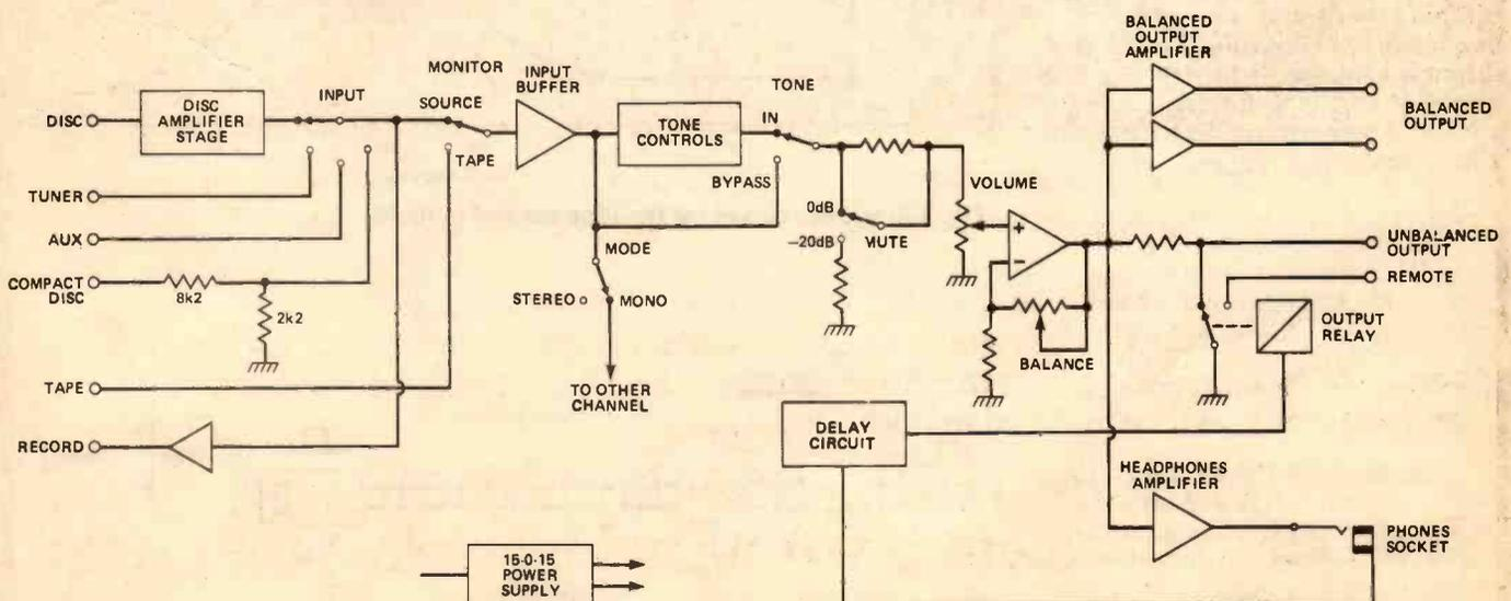
Fig. 1 Block diagram of the extended preamp.
