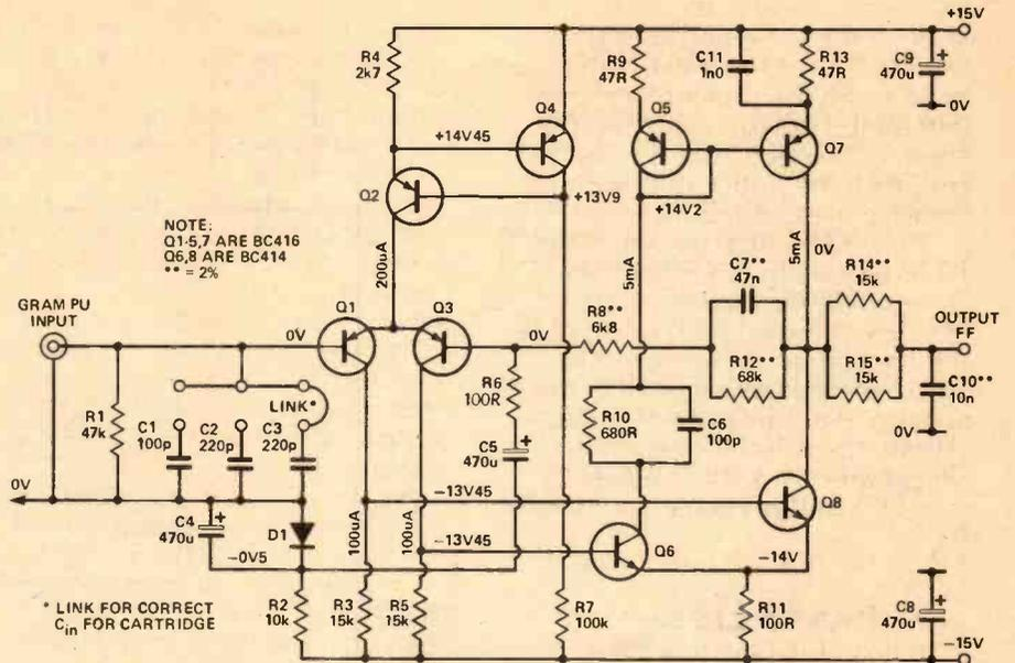
Fig. 3 Full circuit of the PU input stage; note that if you're cutting costs by using 5% resistors, components marked with \*\* must be 2% or better.
