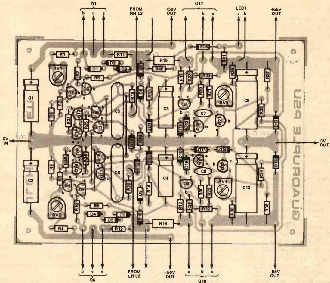
Fig. 9 Overlay diagram for the PSU.
