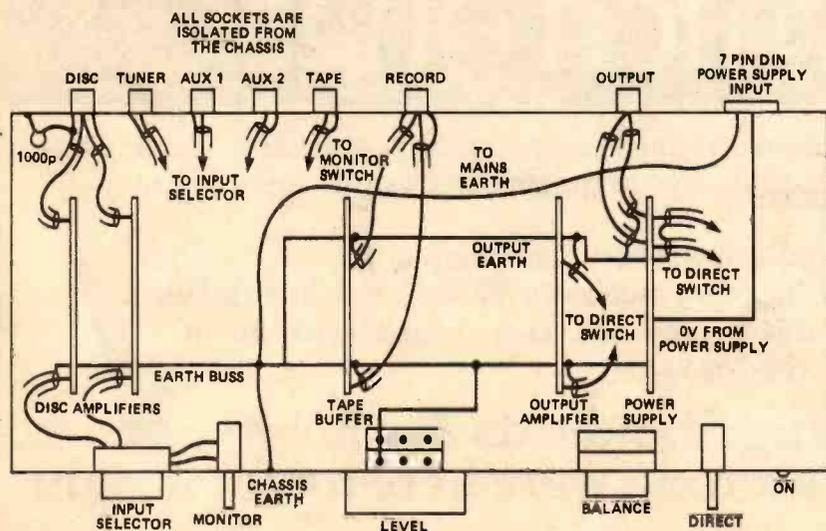
Fig. 11 A possible earthing arrangement.
