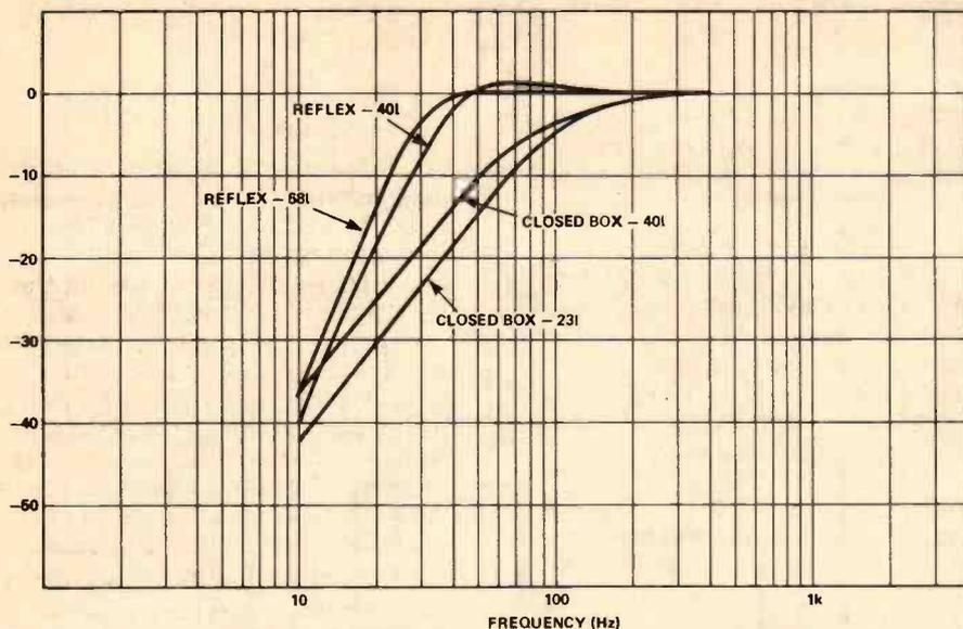
Fig. 1 LF response of the Kef B200G in optimum sized enclosures and in the Active-8 cabinet.
