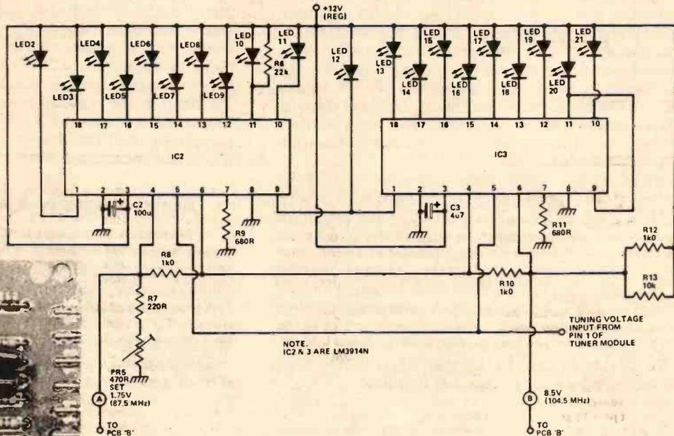
Fig.2 Circuit diagram of the 20 LED frequency scale. This circuit is driven by the tuner module (with its ancillary components) and so the component numbering follows on from the module.
