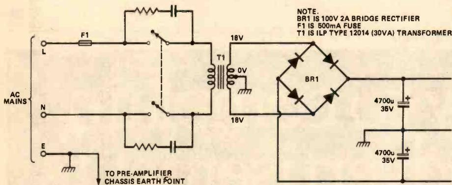
Fig. 10 Suggested circuit to feed the regulated power supply.
