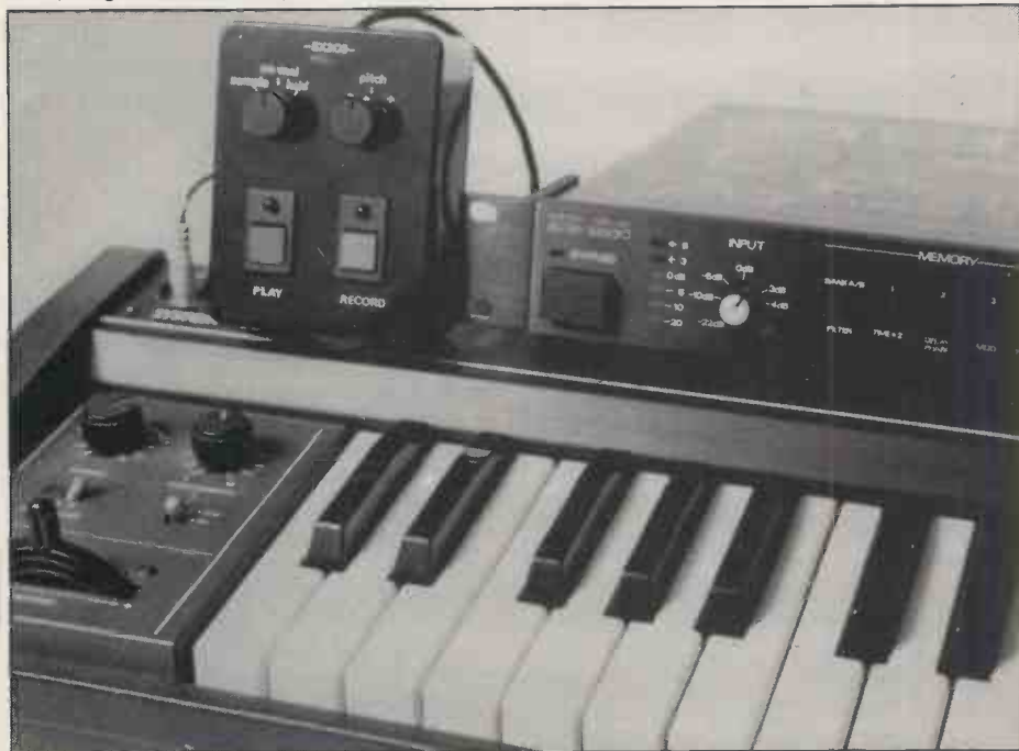
Prototype SX303 being used in conjunction with Roland SDE3000 delay and System 100M controlling keyboard.
