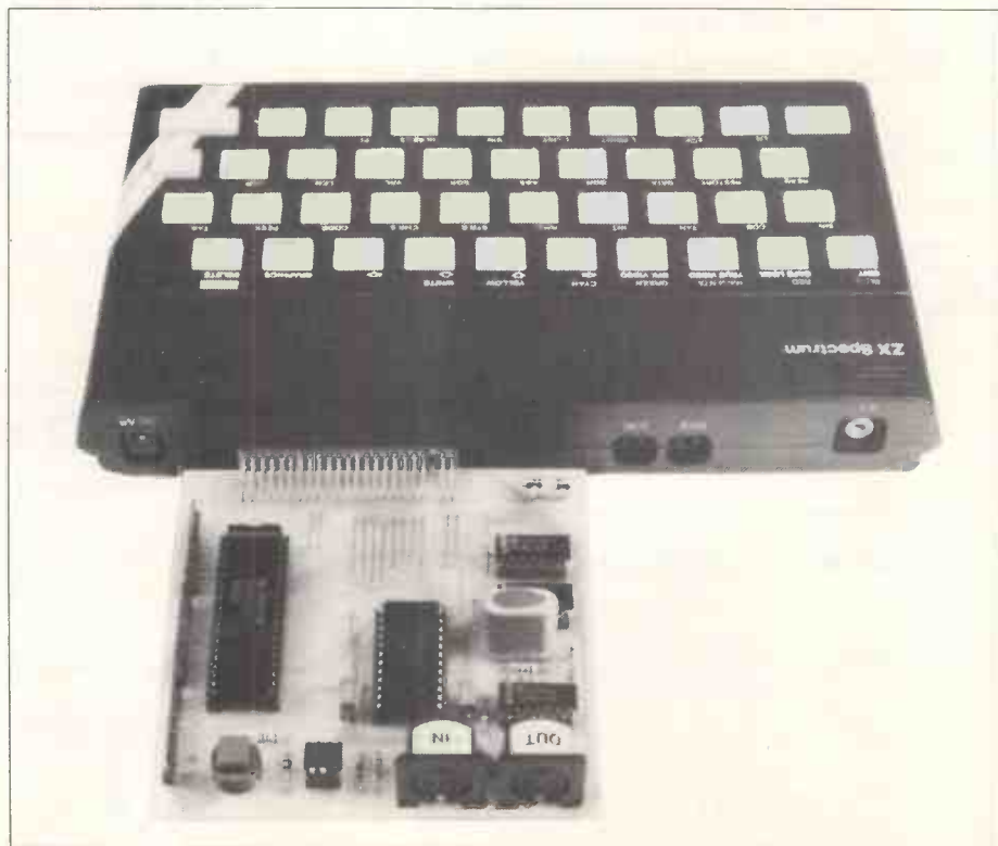
MicroMIDI connected to the Sinclair Spectrum.
