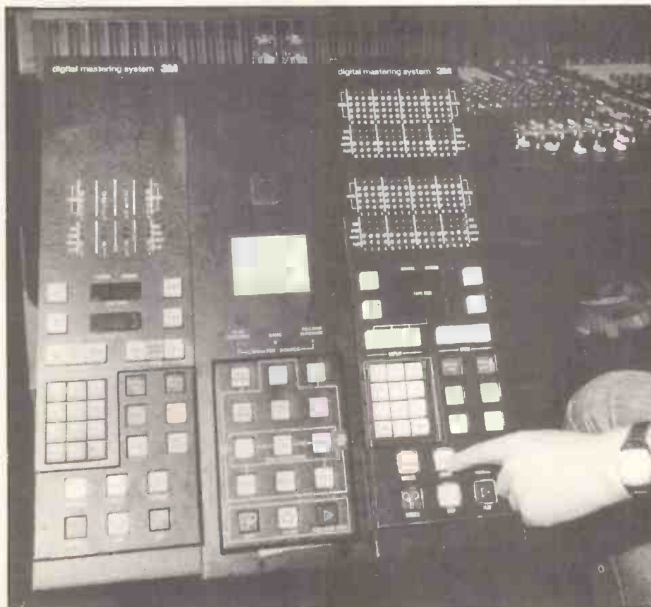
This control panel makes the razor blade and sticky tape redundant. Using the 3M system, an edit can be rehearsed and refined by as little as a millisecond.
