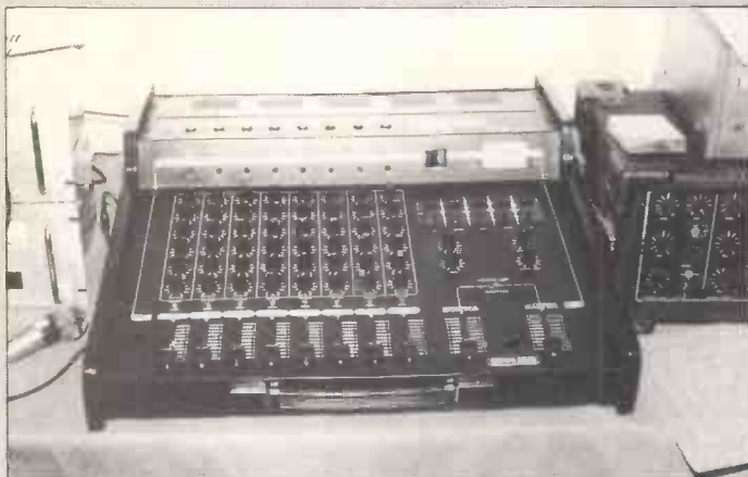
The Custom Sound 701 is an 8 channel powered mixer with graphic EQ. It is available in two power outputs — 150W and 300W.
