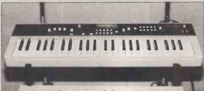
The Casiotone MT-70 is an innovative instrument with two memory storage methods — a bar code reader that picks up scores from a special musical score card, and a manual memory for storage from the keyboard with 10 auto rhythms and 20 presets.
