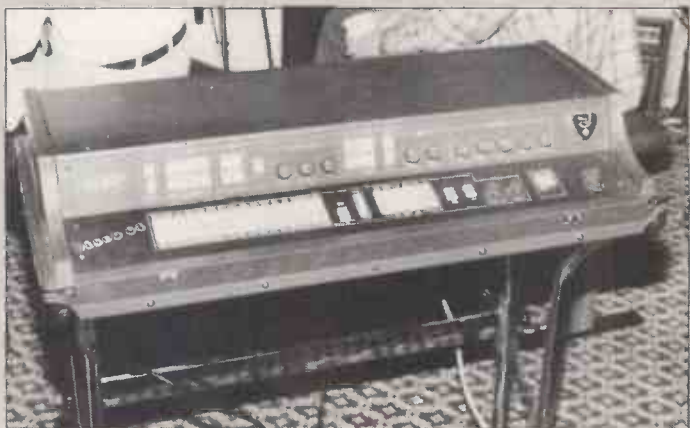
The Solton Disco 64 has as the name implies, 64 preset rhythms utilising 12 voices/effects. 6 keyboard presets and a programmable pedalboard.
