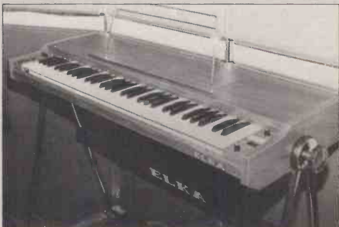
Elka Micropiano 16. This instrument has piano, honky tonk and clavichord effects plus a three track sequencer capable of memorising 128 notes per track.
