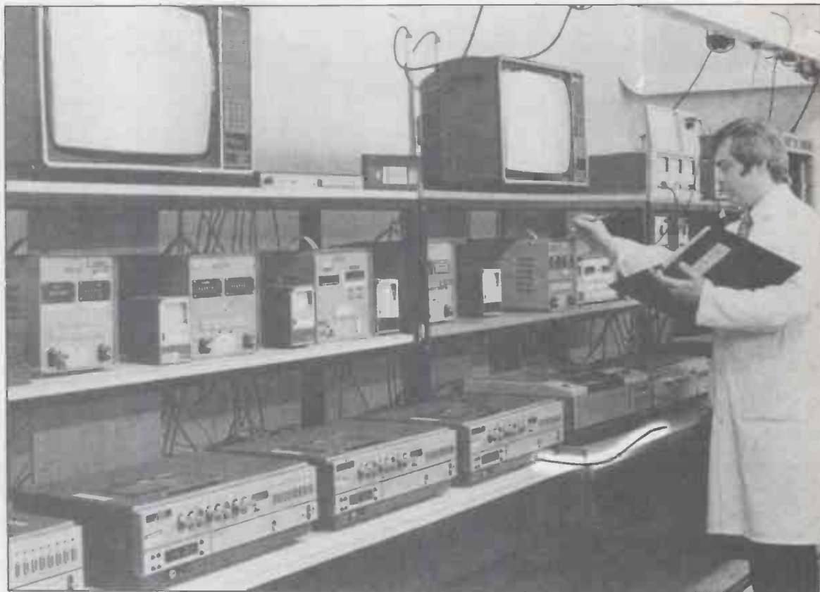
VHS and Beta video cassettes under test in the quality control laboratory at 3M.
