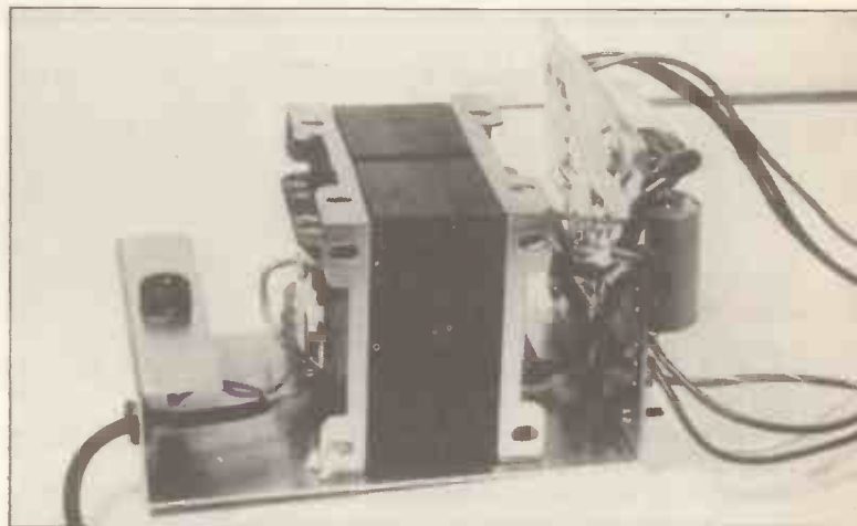
Completed power supply unit.
