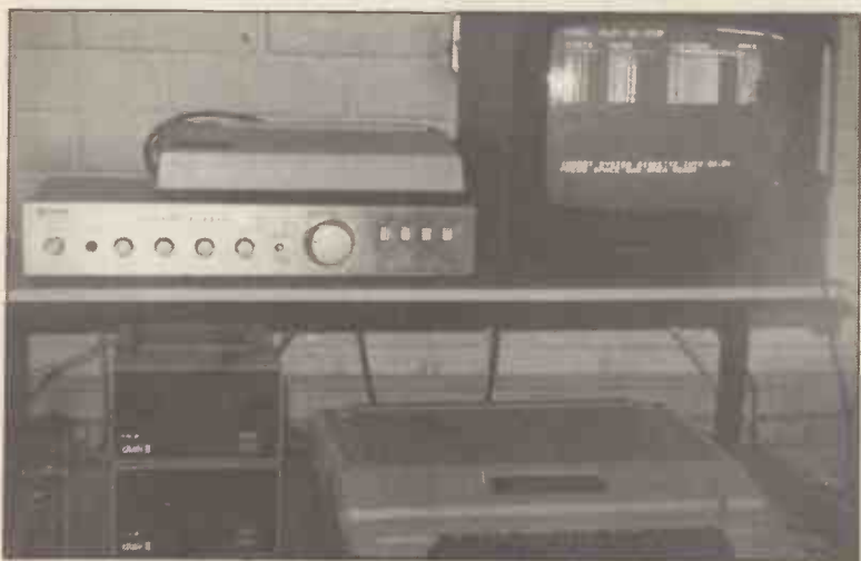
Figure 1. The complete Apple Music System comprising 48K Apple II, MH Music System (light pen included), 2 Disc Drives, Silentype Printer and VDU.
