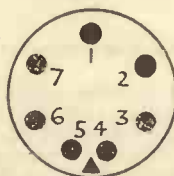
This diagram shows the arrangement of the pins on the bases of valves made by members of the British Radio Valve Manufacturers Association. The bases are (left to right) four, five, seven and nine pin types. The numbering of the pins corresponds with the table below, and the code in the table is explained at the top of this page.
