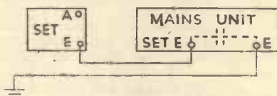
FIG. 12.—Essential safety condenser for the earth connection of a D.C. mains unit.
