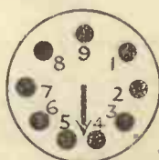
This diagram shows the arrangement of the pins on the bases of valves made by members of the British Radio Valve Manufacturers Association. The bases are (left to right) four, five, seven and nine pin types. The numbering of the pins corresponds with the table below, and the code in the table is explained at the top of this page.
