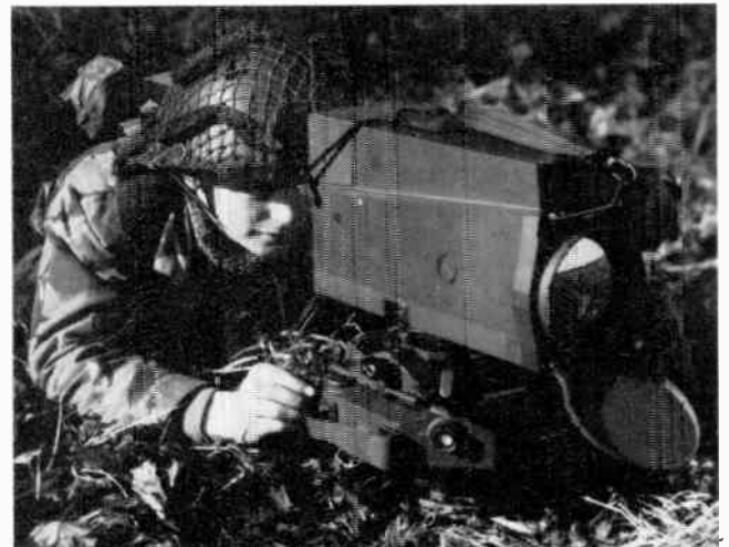
Fig. 24. A complete thermal imager using Class 1 modules from the MOD Thermal Imaging Common Modules Programme produced by EMI Electronics.
