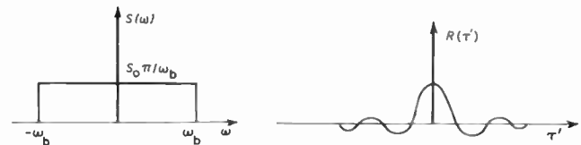
Fig. 4. Power spectrum and autocorrelation of the input signal x(t) .
