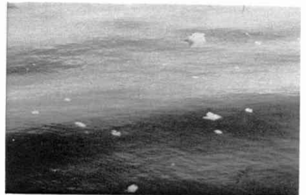
Fig. 8. Swell 5 ft. Sea crystalline (-5°C). Ribbon ice at 1.5 n.m. Wind force 2. First detected at 12 n.m. and 4 n.m. on high and low resolution sets respectively.
