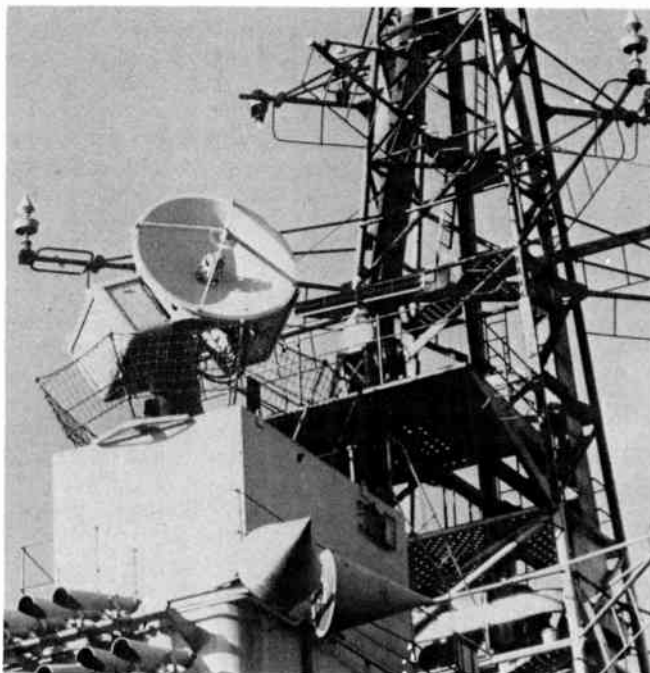
Fig. 1. Skynet V aerial head fitted on RN ship.
