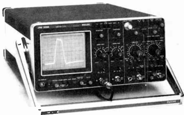
Fig. 1. Philips new 100 MHz PM 3266 storage oscilloscope uses a transfer charge tube system to provide high writing speeds up to 1000 div/ \mu s with display over the whole screen
