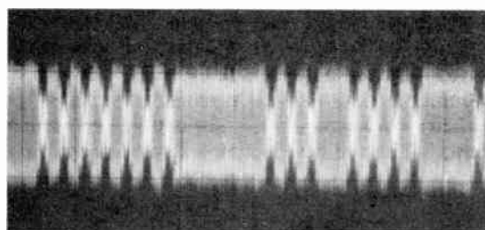
(b) Expanded section of the impulse response (0.25 \mu\text{s}/\text{div} ).
